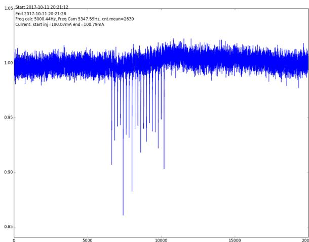
Figure 1: Drop in relative intensity during injections measured at beam line P07 [2]. The time duration is 16 seconds.
