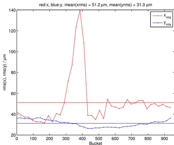
Figure 3: RMS value of injection transients by kicker magnets for different bunch positions in the filling pattern.
