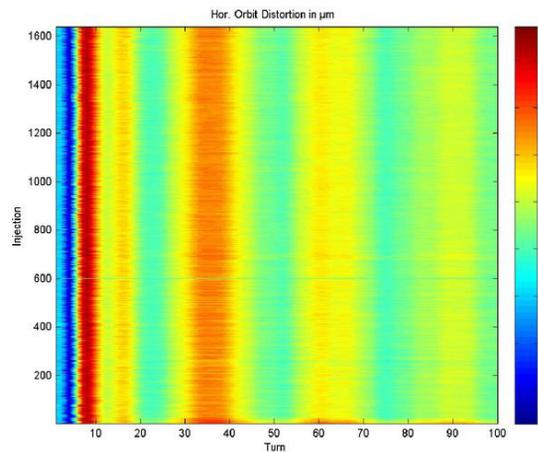
Figure 5: Stability of the horizontal injection oscillations measured for 100 turns after injection for 1600 injections which corresponds to a duration of 20 h. The deviations in  $\mu\text{m}$  are coded in different colors.
