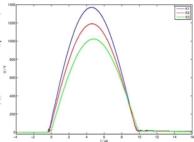
Figure 2: Pulses of the three injection kickers.
