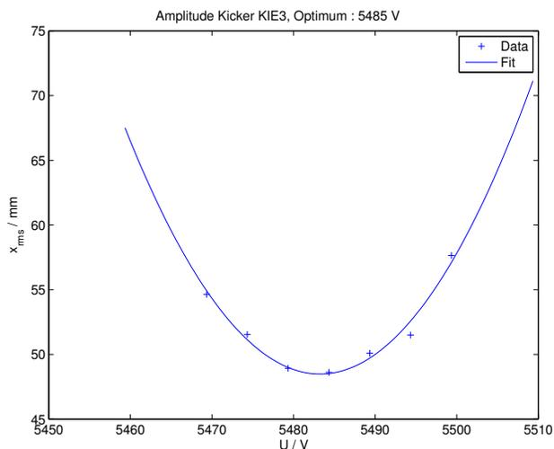
Figure 4: Parameter scan of one of the kicker voltages.
