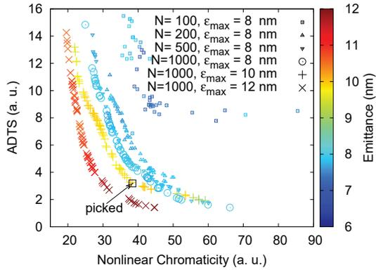
Figure 2: Pareto fronts evolution and the results with different emittance limits.
