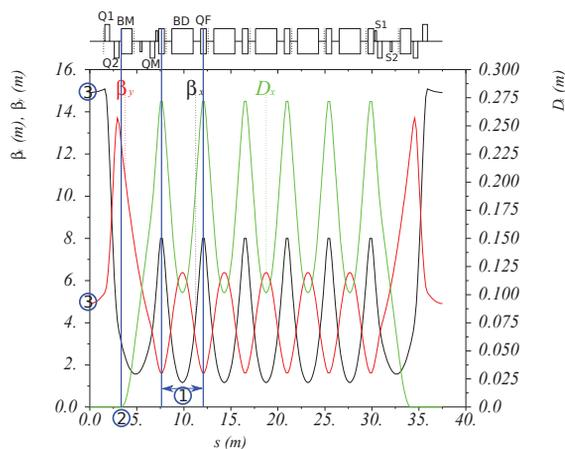
Figure 1: Lattice schematic and the naming convention.
