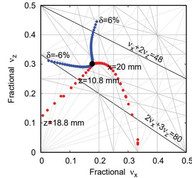
Figure 4: Tune spread envelopes in the tune diagram.
