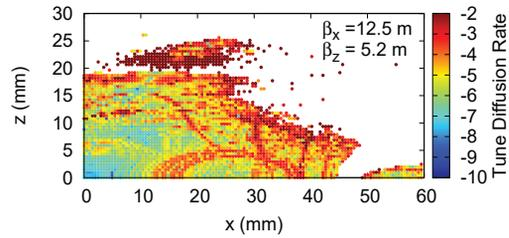
Figure 3: On-momentum dynamic aperture without errors.
