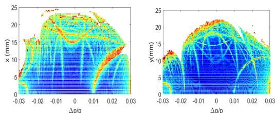
Figure 3: MA at the centre of long straight section. (Left) horizontal plane; (right) vertical plane.
