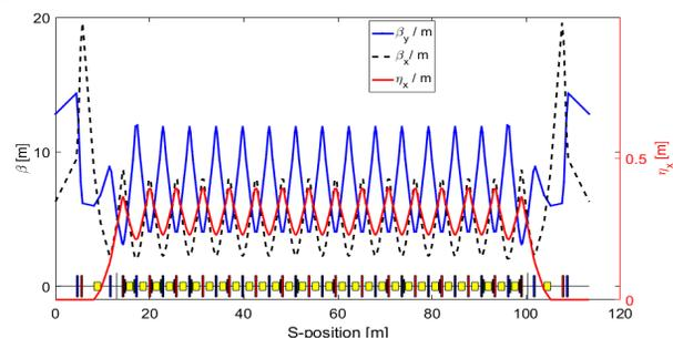
Figure 1: Layout of a quarter of the booster lattice.
