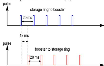
Figure 5: Pulse separations in the two high energy transport lines.
