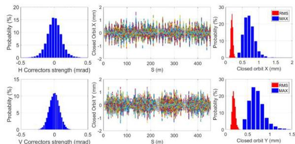
Figure 2: Closed orbit distortion after correction.
