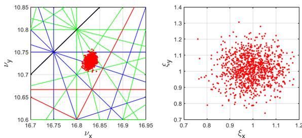
Figure 4: Tune and chromaticity distribution with errors and closed orbit correction.
