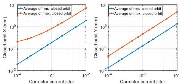
Figure 10: Closed orbit with different corrector current jitter.
