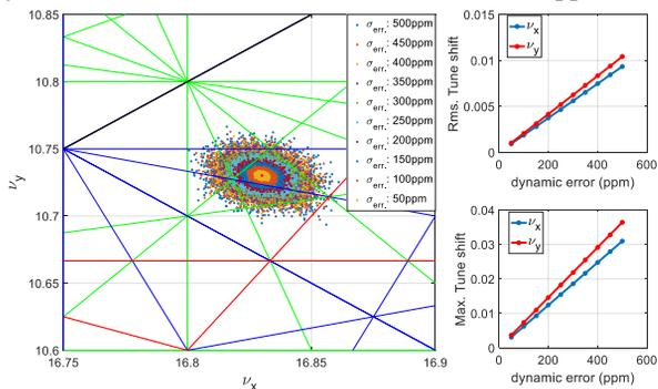
Figure 8: Tune spread with different dynamic errors.
