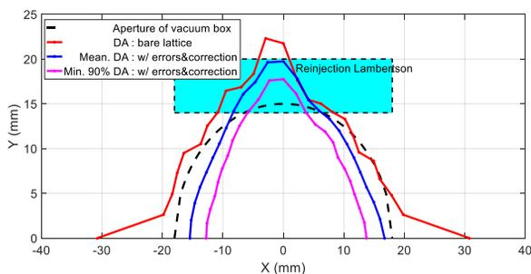
Figure 5: Dynamic aperture of bare lattice (red), average DA (blue) and minimum case of 90% confidence DA (purplish red) with errors and correction and aperture of vacuum box (black).
