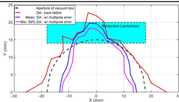
Figure 7: Dynamic aperture of bare lattice (red), average DA (blue) and minimum case of 90% confidence DA (purplish red) with multipole errors and aperture of vacuum box (black).
