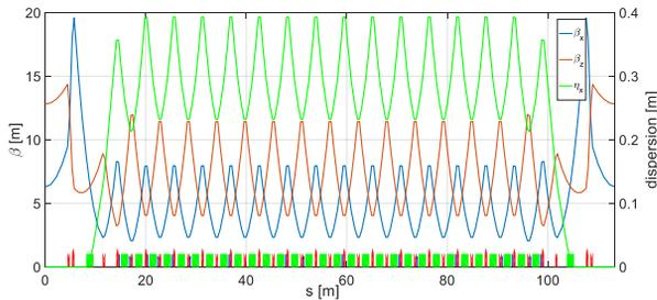
Figure 1: Optical functions and layout of one super-period lattice of the HEPS booster.
