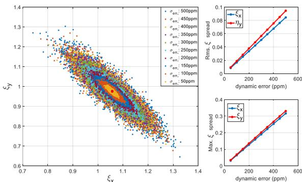
Figure 9: Chromaticity spread with different dynamic errors.
