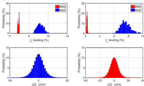
Figure 3: Beta beating (top) and residual dispersion distribution (down) with errors and closed orbit correction.
