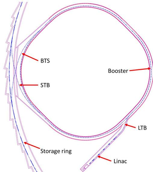
Figure 1: Layout of the HEPS injector.
