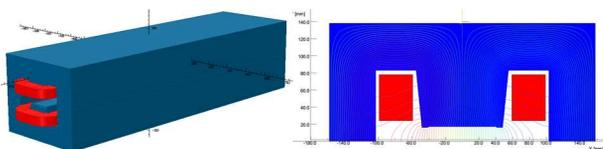
Figure 4: The physics model of the booster dipole.
