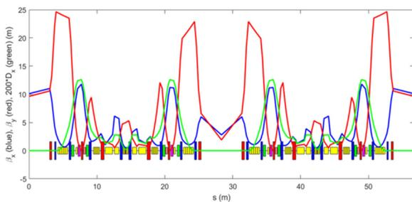
Figure 2: Optical functions and layout of one period (two 7BAs) of the 34-pm lattice.
