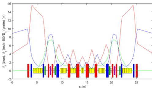
Figure 1: Optical functions and layout of one 7BA of the 58-pm lattice.
