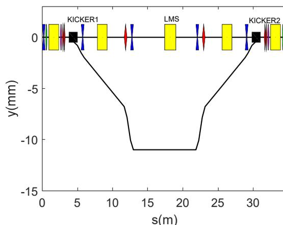
Figure 3: The layout and beam trajectory of the injection system from the storage ring.
