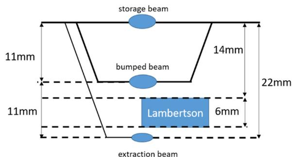
Figure 5: The schematic at the entrance of lambertson for the extraction section.
