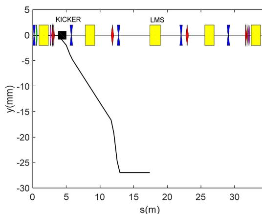
Figure 1: The schematic layout of the injection scheme of the booster.
