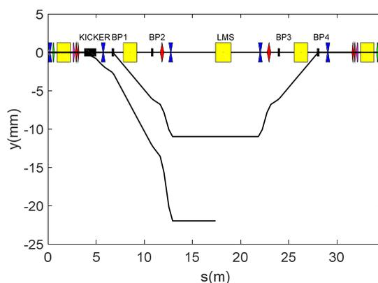
Figure 4: The layout and beam trajectory of the extraction system.
