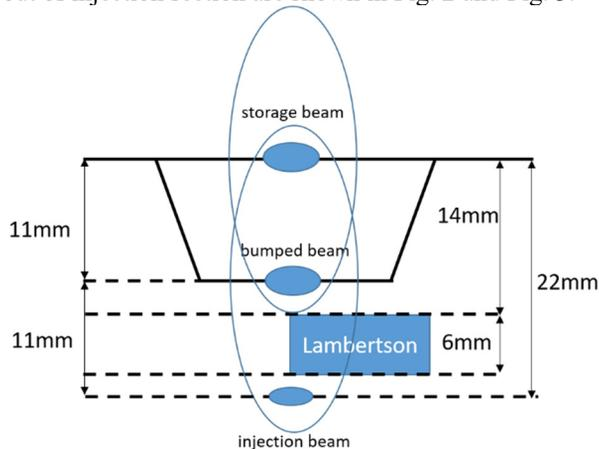
Figure 2: The schematic at the exit of lambertson for the injection system from the storage ring.
