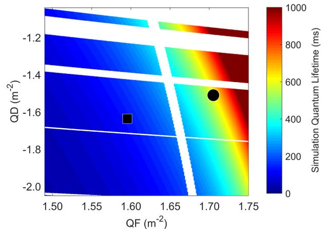
Figure 3: Simulation quantum lifetime for a quadrupole scan at 2.9 GeV with  $V_{rf} = 1.75$  MV. The commissioning optics are marked with a black square and the design optics are marked with a black circle.
