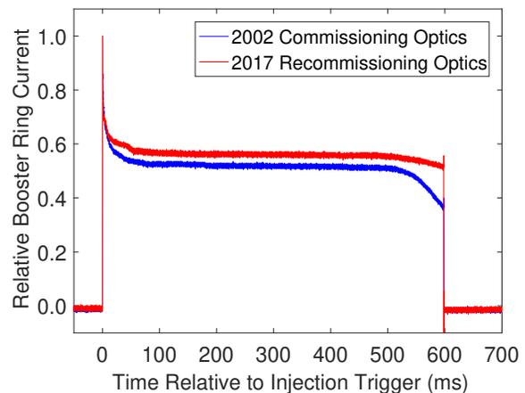
Figure 4: Current profiles over one booster ramp showing the approximately 6% current loss at extraction energy with the recommissioned optics, which are similar to the design optics, compared with the approximately 25% current loss with the original commissioning optics.
