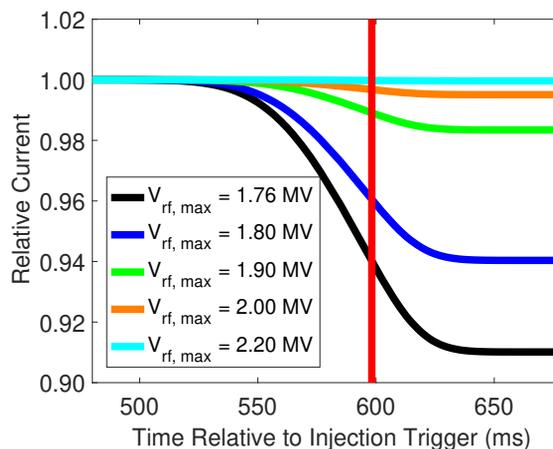
Figure 7: Comparison of simulated booster current profiles with increased  $V_{rf,max}$  with the extraction time marked with a red line.
