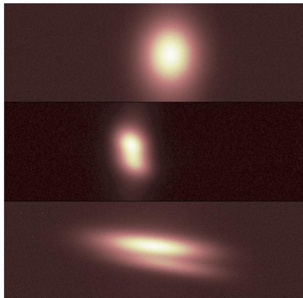
Figure 6: Observation of the booster beam using the synchrotron light monitor at 25  $\mu$ s after injection (top), 220 ms after injection (middle) and 592 ms after injection (bottom), which is the time of extraction. The vertical distortion to the middle image and the artifact in the bottom image are believed to be due to radiation damage to the prism.
