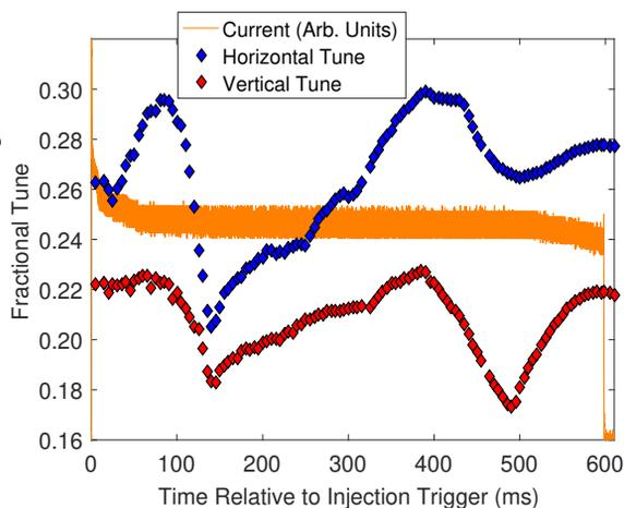
Figure 5: Measured tune drift over the ramp plotted with the measured current profile after recommissioning.
