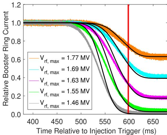
Figure 2: Comparison of measured booster current (colored data) with calculations based on quantum lifetime (black curves) for various  $V_{rf,max}$  with the extraction time marked with a red line.
