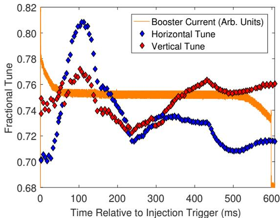
Figure 1: Measured tune drift over the ramp plotted with the measured current profile with the original commissioning optics.
