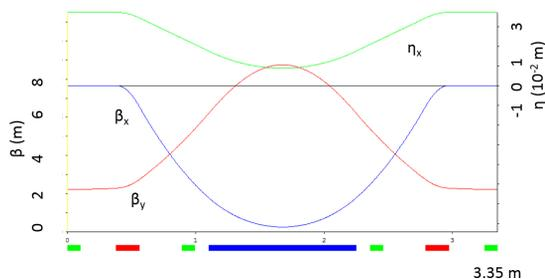
Figure 4: Unit cell with tune advances set to  $\Delta v_x = 3/7$  and  $\Delta v_y = 1/7$ .
