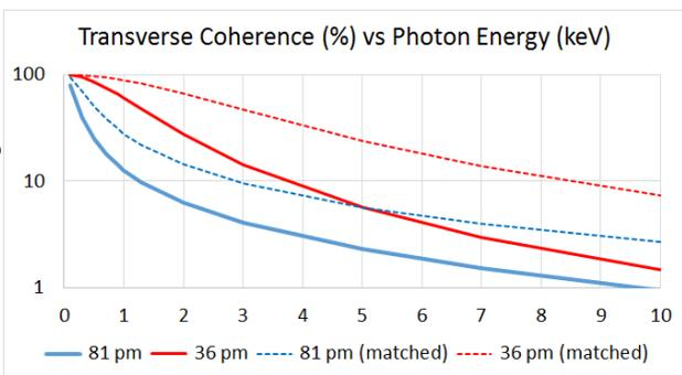
Figure 9: Transverse Coherence for the 81 pm and 36 pm MBAs. ID length is 4 m and vertical coupling is 1 %.
