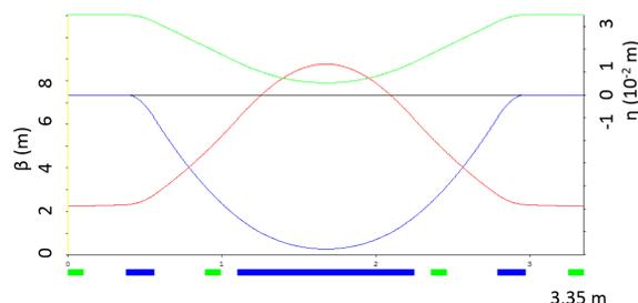
Figure 7: Unit cell with quadrupoles replaced by reverse bends. A reduction of dispersion in the main dipole results.
