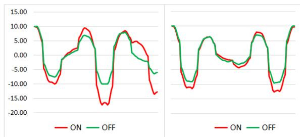
Figure 3: Tracking through 7 cells starting from a horizontal offset of 10 mm with sextupoles ON and OFF. Left:  $\Delta v_x = 2.5$ ; Right:  $\Delta v_x = 3.0$ .
