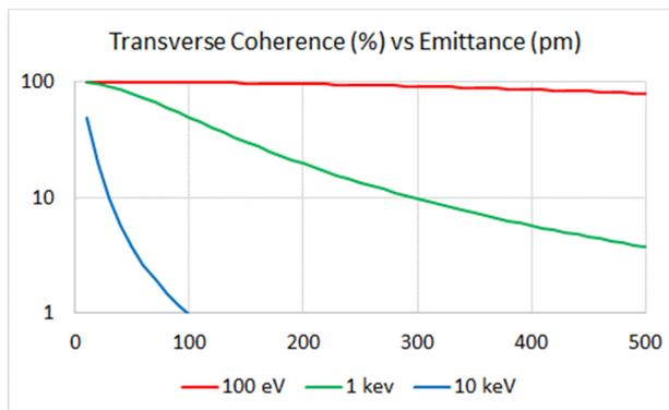
Figure 1: Transverse coherence vs electron emittance for three photon energies. (The electron and photon phase spaces are assumed to be matched. The vertical coupling is 1 %.)
