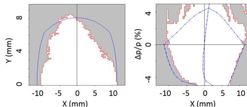
Figure 6: DA (left) and MA (right) for the MBA.
