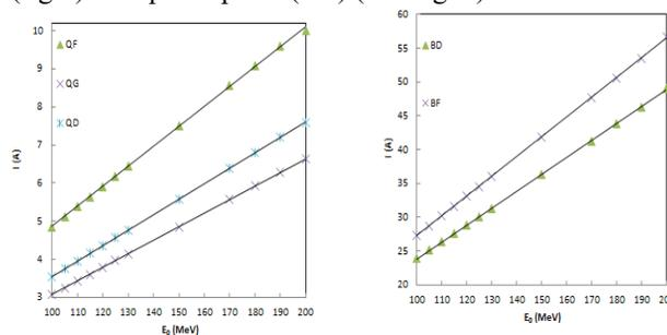
Figure 1: Booster dipole current of BD (green) and BF (black) at different injection energy (right); booster quadrupole current of QF (green), QD (cyan), and QG (black) at different injection energy (left).
