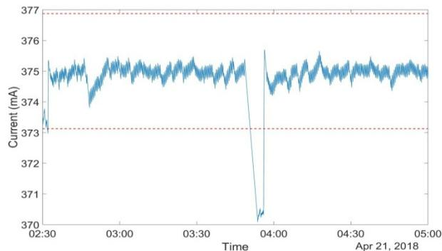
Figure 5: Storage Ring Current during top off with 100 MeV booster injection. The horizontal lines show  $\pm 0.5\%$  of the nominal current.
