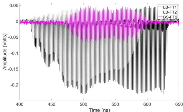
Figure 2: Bunch Pattern from injector during 100 MeV operation. The color code matches Figure 1. The horizontal position of the grey and magnet trains are aligned manually relative to the black. storage ring.
