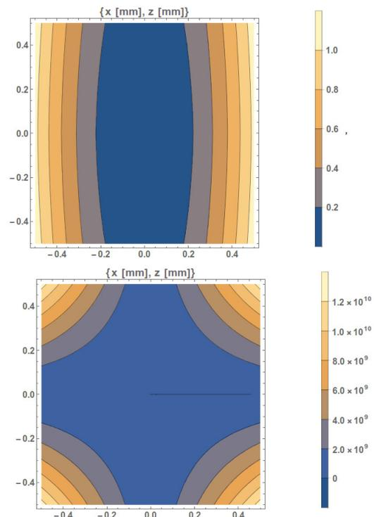
Figure 3: Map of values of  $K_x$  and  $K_z$  in values relative to the deviation of the value in the central trajectory, in percentage, in the vertical polarization of Delta21 (See [8]).
