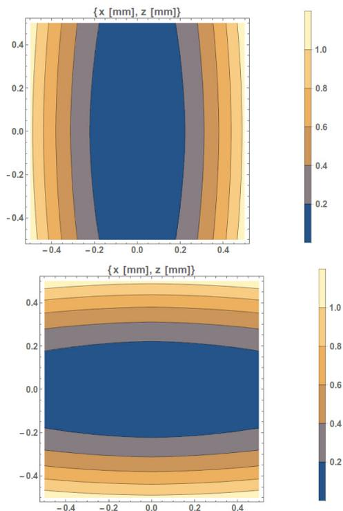
Figure 4: Map of values of  $K_x$  and  $K_z$  in values relative to the deviation of the value in the central trajectory, in percentage, for the circular polarization of Delta21 (See [8]).
