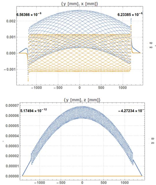
Figure 1: Trajectory with angles correction for  $x = 0.3$  mm and  $z = 0.2$  mm compared to the central orbit in the vertical polarization of the undulator Delta21 (See [8]).
