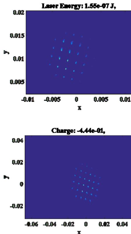
Figure 2: A typical laser image (top) and corresponding electron beam image. The maximum laser beam size is limited by the UV camera aperture. The scale is in meters.
