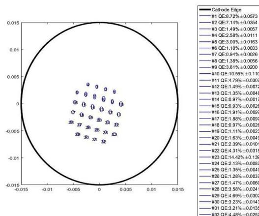
Figure 3: A QE map produced by this method with a 32 beamlet array. The scale is in meters.
