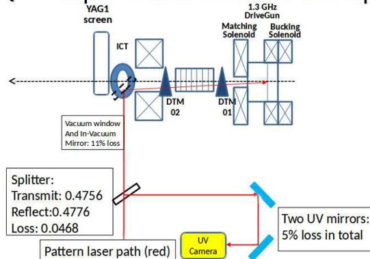
Figure 1: Schematic of the experimental setup. The laser path begins AFTER the MLA optics.
