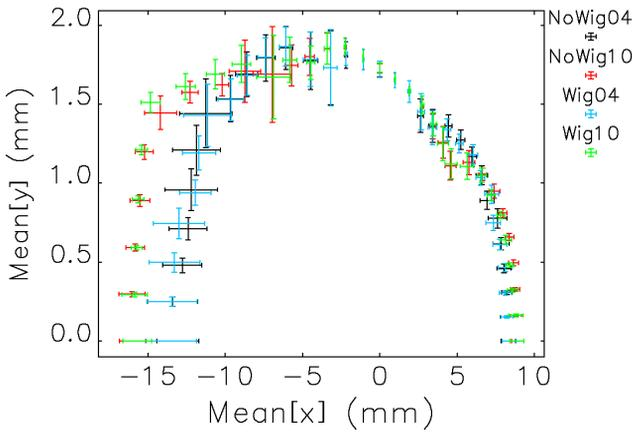
Figure 4: Calculated DA for error sets with (Wig04 and Wig10) and without (NoWig04 and NoWig10) measured HSCU multipole errors.
