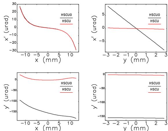
Figure 2: On-axis kickmap before (HSCU0) and after (HSCU) local correction.
