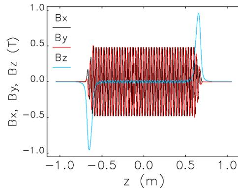
Figure 1: Calculated on-axis HSCU field.
