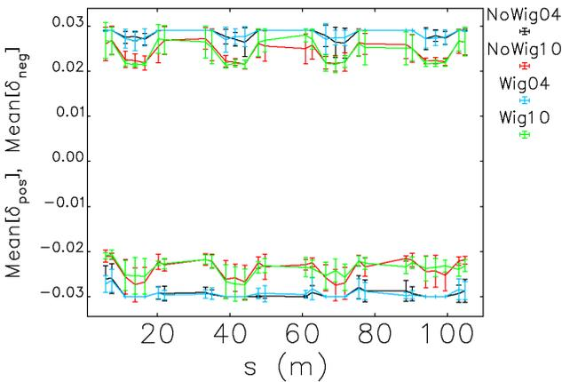
Figure 5: Calculated LMA for error sets with (Wig04 and Wig10) and without (NoWig04 and NoWig10) measured HSCU multipole errors.
