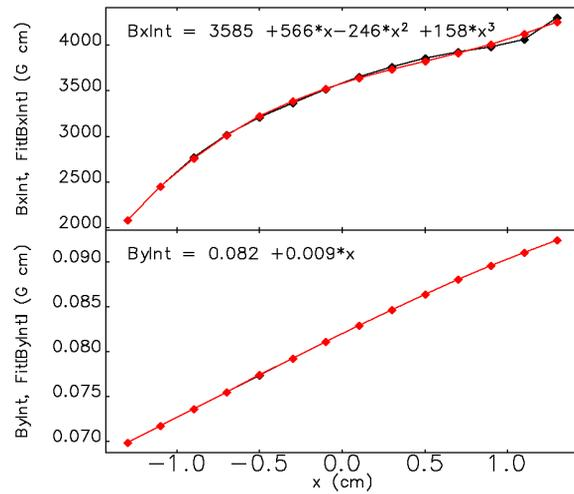
Figure 3: Calculated field integral vs  $x$  at  $y = 0$  from field map. The fitted multipole components agree well with the kickmap calculation results, see Table 2. This means the major contribution to the calculated kickmap is the non-vanishing field integrals, and not the beam orbit wiggling inside the device.
