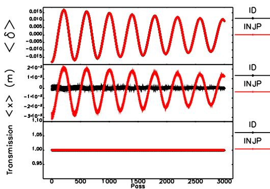
Figure 6: Bunch centroid and transmission parameters. ID: nominal ID; INJP: injection ID ( $D_x=0.15$  m).
