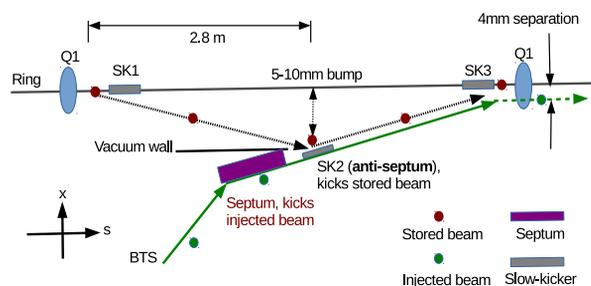
Figure 2: Sketch for synchrotron accumulation on off-energy closed-orbit with anti-septum [4] in 3-slow-kicker scheme. APS-U example in one 5.8 m ID.
