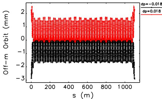
Figure 5: Off-energy closed-orbit of beam with energy offset of  $\pm 1.8\%$ . Starting point is injection ID center.
