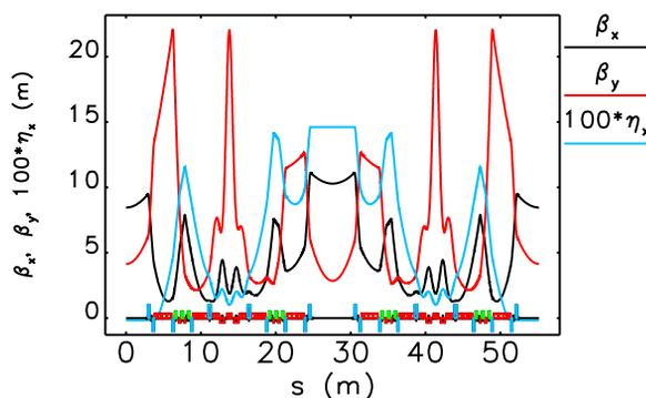
Figure 3: High horizontal dispersion ( $D_x=0.15$  m) injection ID. Blue blocks represent quadrupoles, red blocks represent dipoles, and green blocks represent sextupoles.
