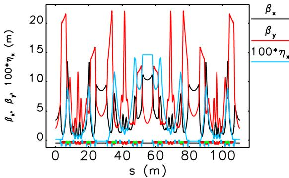
Figure 4: Two alternating-beta APS-U storage ring sectors, plus these 2 sectors near the injection ID straight.
