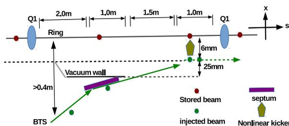
Figure 1: Sketch for synchrotron accumulation on off-energy closed-orbit with a single pulsed nonlinear kicker. APS-U example in one 5.8 m insertion.
