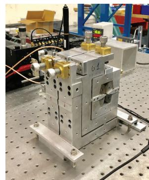
Figure 8: Two quadrupoles representing one quadrupole wiggler period on the magnetic measurement bench.
