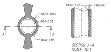
Figure 5: The design of the corrugated waveguide.
