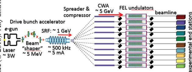
Figure 1: A schematic of the facility showing up to ten individual CWAs, FELs and beamlines.
