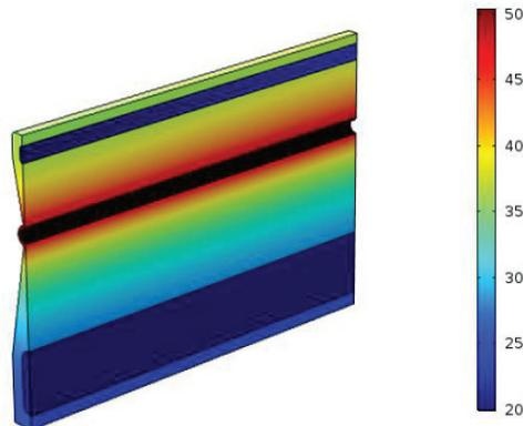
Figure 4: The vacuum chamber with the corrugated waveguide (half of the chamber is shown). The temperature distribution is shown in degrees Celsius.
