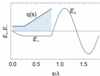
Figure 2: Electron charge distribution  $q(s)$  proposed in [5] shown as a filled area; the corresponding accelerating and decelerating field shown by the blue curve.
