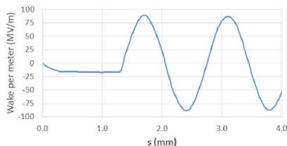
Figure 6: The wake potential function for 10 nC drive bunch calculated with ECHO code [8].
