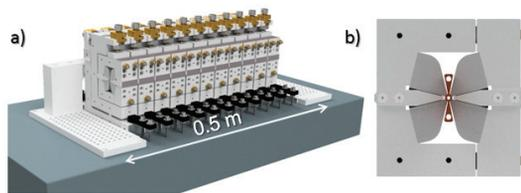
Figure 3: An accelerator module and a front view on the permanent magnet quadrupole and the vacuum chamber.
