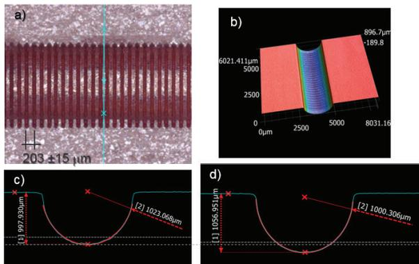
Figure 7: A segment of one half of the corrugated waveguide: a) image under the microscope, b) digital rendering, c) cross-sectional profile through a raised tooth marked by the light blue line in a), and d) cross-sectional profile through a groove.
