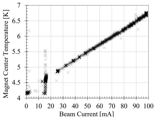
Figure 8: Magnet temperature plotted against circulating e-beam current during initial machine start-up.
