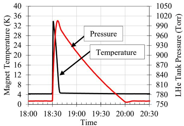
Figure 5: HSCU quench recovery. Magnet temperature spikes comparatively quickly while reservoir pressure decreases gradually over 1.5 hour.
