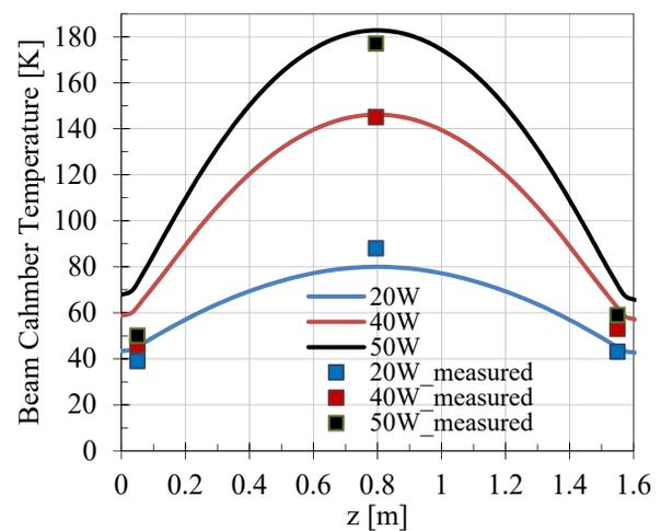
Figure 6: Beam vacuum chamber temperature along chamber length for three different heat dissipation levels. Solid curves are calculation, points are measured data.
