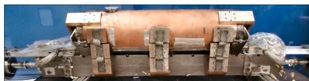
Figure 3: HSCU cold mass assembly including magnet, beam vacuum chamber, and liquid helium reservoir.
