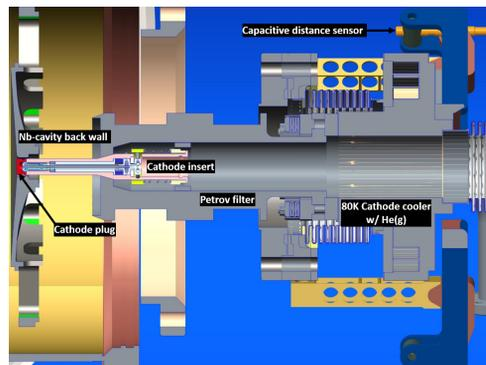
Figure 4: Cross section through the gun cavity - cathode interface region.
