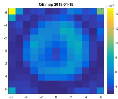
Figure 7: QE map (12 mm × 12 mm) of the Cu photocathode inside the gun. The diameter of the plug is 10 mm and the laser spot size was 1.9 mm. A QE of in range of  $10^{-5}$  was measured over the whole area.
