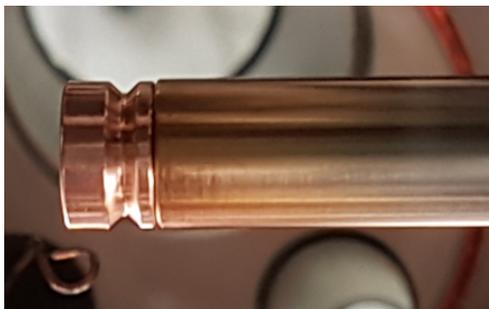
Figure 3: The cathode insert based on the HZDR-design with the exchangeable plug before insertion into the SRF-gun module. The bulk Cu plug is used as the photocathode for commissioning purposes for RF-operation and first electron beam. The color changes of the Cu-insert are due to the bake out of the transfer system for vacuum commissioning.
