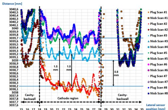
Figure 6: Laser distance measurement of the photocathode position with respect to the Nb-cavity back wall before and after alignment. The relative distances are in agreement with the signals of the capacitive distance sensors at the cathode cooler.
