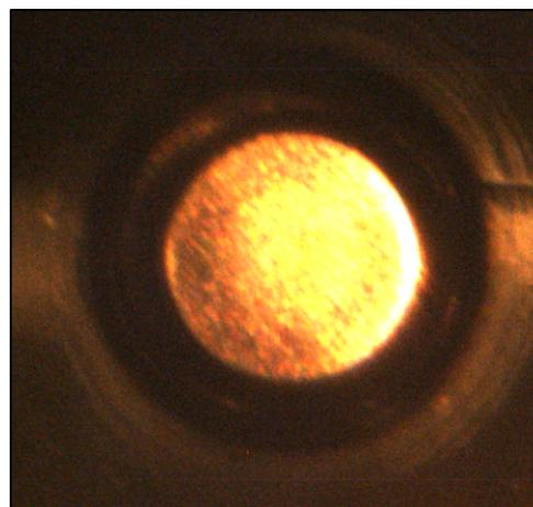
Figure 5: Camera image of the Cu plug after successful insertion into Gun 1.0 cavity.
