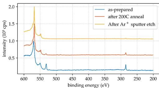
Figure 2: XP spectra (Al  $K\alpha$ ) including the Cu LMM Auger transitions ( $> 540$  eV), O 1s (531 eV), C 1s (285 eV) peaks taken after each preparation step.
