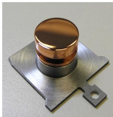
Figure 1: The flag style sample holder system with the polycrystalline Cu plug used as a photocathode for initial commissioning of the SRF-Photoinjector. The diameter of the plug is 10 mm.
