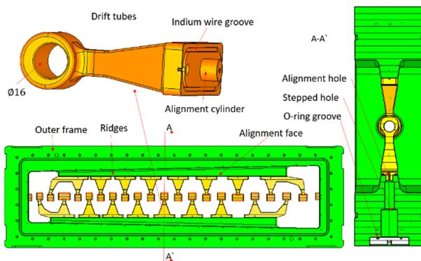
Figure 2: Schematic drawing of the central frame.
