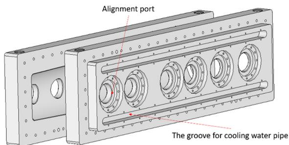
Figure 3: Schematic drawing of the tank half shells.
