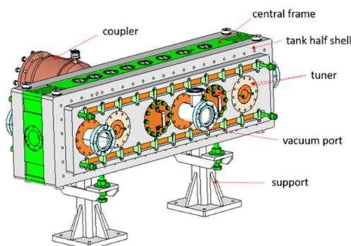
Figure 1: Assembly view of the IH DTL.
