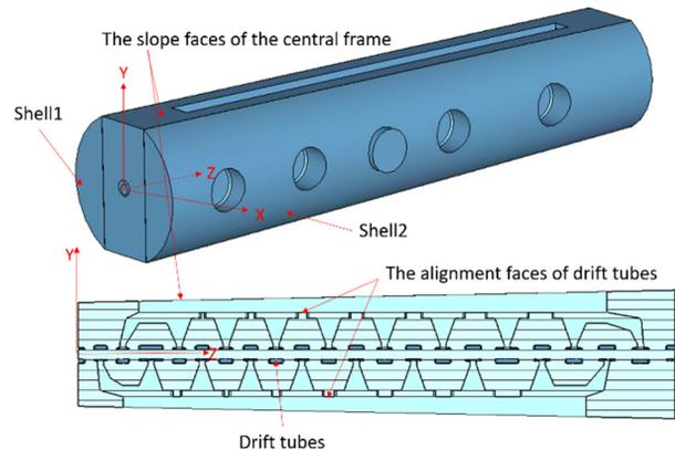
Figure 4: A CST model of IH-DTL for error analysis.
