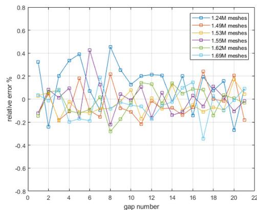
Figure 5: Relative error of CST simulation for different meshes.
