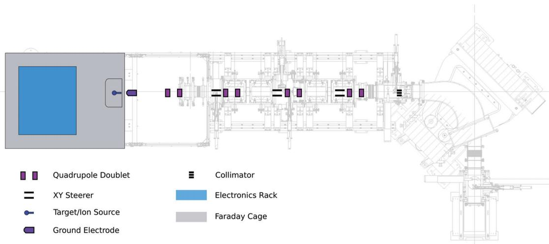
Figure 3: The basic layout of the ARIEL optics between the ion source (here a surface ion source is used) and the pre-separator magnet, overlaid on a drawing of the OATIS beam line.
