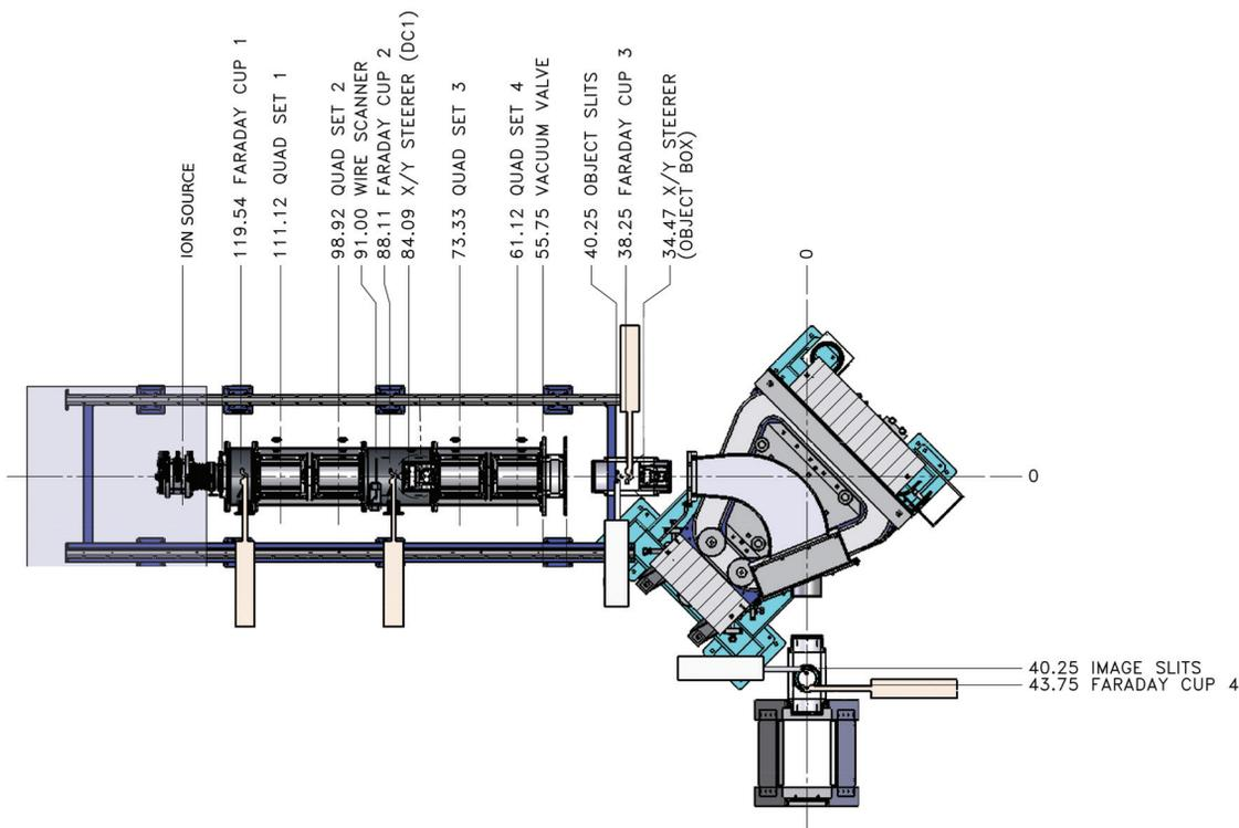
Figure 1: Layout of the current OATIS test stand, showing the ion source and the separator magnet, as well as the locations of 4 Faraday cups, 4 sets of quadrupoles, 2 XY steerers, a wire scanner and 2 sets of slits. The position of each element relative to the origin at the 90° magnet is given in inches before the element name.
