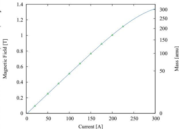
Figure 2: Magnetic field as a function of current in the coils for the OATIS separator magnet, measured at the magnet midplane. The mass theoretically able to be transported with this magnetic field is shown on the right.
