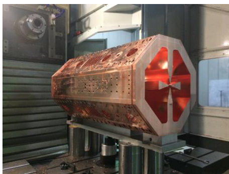
Figure 3: Post-processing of the brazed segment #2.
