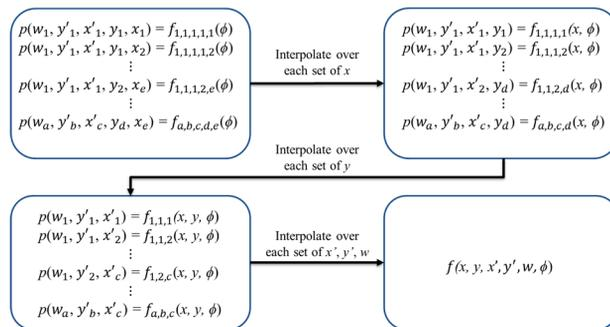
Figure 5: Scheme for proposed 6D interpolation.
