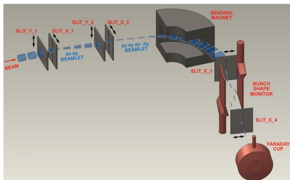
Figure 1: A diagram showing the concept of a full six-dimensional emittance scan.
