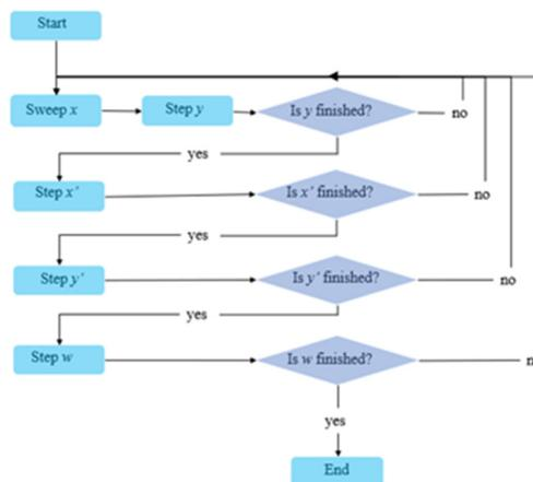
Figure 3: A diagram showing the logic behind the 6D scan.
