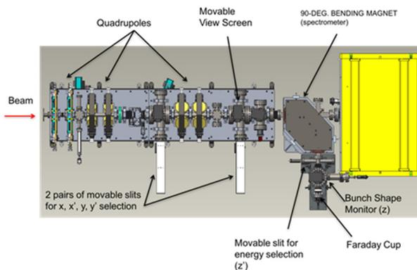
Figure 2: A schematic view of the BTF MEBT which contains the diagnostics for the 6D scan.
