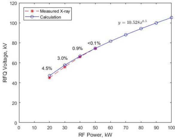
Figure 4: RFQ vane voltage calibration results.
