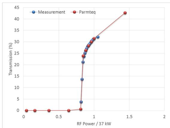
Figure 5: Comparison between measured and calculated RFQ transmission for  $^{40}\text{Ar}^{9+}$ . Power normalized on 37 kW.
