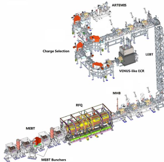
Figure 1: FRIB Front End layout. Two ECR ion sources (ARTMIS and VENUS-like ECR) are located at the ground level. The MHB, RFQ and MEBT are located in the linac tunnel 10 m below grade.
