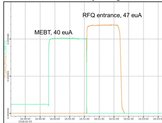
Figure 6: Transmission of  $^{40}\text{Ar}^{9+}$  beams through RFQ with MHB.
