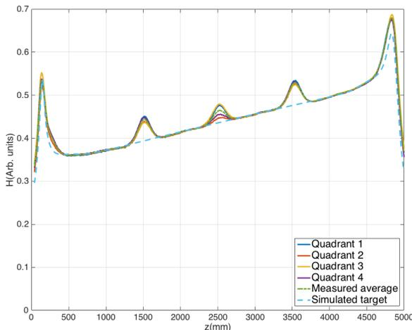
Figure 2: Final RFQ bead-pull measurement showing the magnetic field profiles of the four quadrants.
