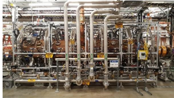
Figure 3: FRIB RFQ installed in beamline with support stand, water cooling manifold, vacuum pump and RF waveguide connected to the input coupler.
