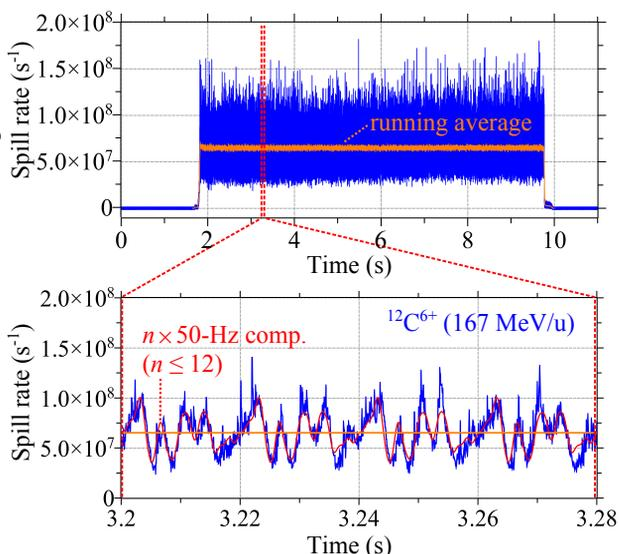
Figure 4: A spill of  $^{12}\text{C}^{6+}$  delivered to a treatment room at constant average intensity (with DIC enabled), measured using the IC at the beam outlet. The approximating red curve is obtained by inverse Fourier transform of the 9 most prominent 50-Hz harmonics as shown in Fig. 5 (top).
