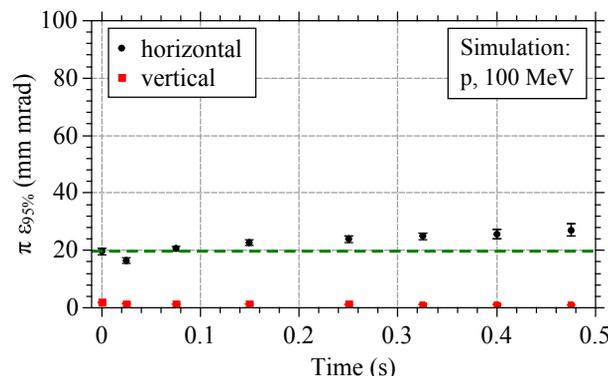
Figure 3: Results from a tracking simulation (p, 100 MeV) of the RF-KO process, optimised for DIC: The KO RF spectrum is shifted towards the extraction resonance (top). Higher RF power is required, but the horizontal emittance of the stored beam is almost unaffected by the extraction (bottom).
