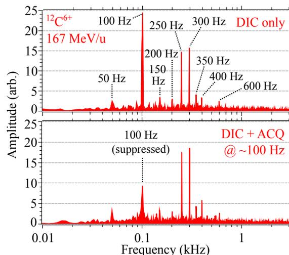
Figure 5: Discrete Fourier transforms (FFTs) of time structures of  $^{12}\text{C}^{6+}$  spills. Top: FFT of the standard spill from Fig. 4, with the most important power-grid harmonics highlighted. Bottom: The otherwise same accelerator cycle, but with the ACQ magnet operating near 100 Hz such as to cancel out the machine-intrinsic modulation at that frequency.
