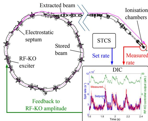
Figure 1: Working principle of the DIC: Ionisation chambers measure the instantaneous spill rate at the beam outlet. A feed-back loop continuously corrects the amplitude of the RF-KO signal such as to meet the intensity set-point of the STCS.
