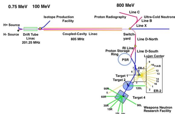
Figure 1: Layout of LANSCE Accelerator Facility.
