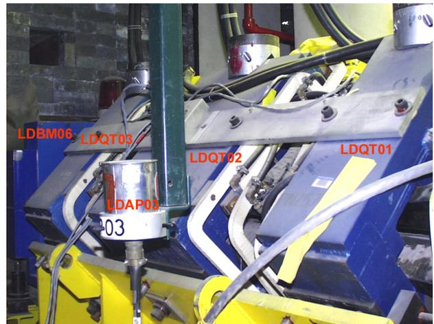
Figure 5: Position of LDAP03 monitor with respect to LDQT01-03 quadrupole triplet.
