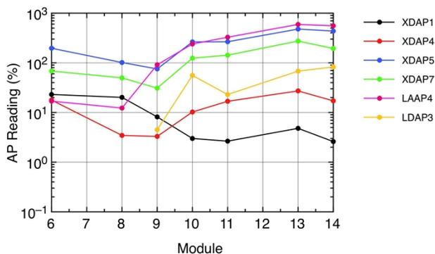
Figure 7: Beam spill normalized by 1% variation in RF amplitude.
