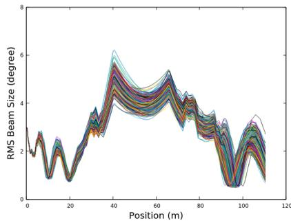
Figure 7: The Z direction rms beam size results in the errors and correction scheme study.
