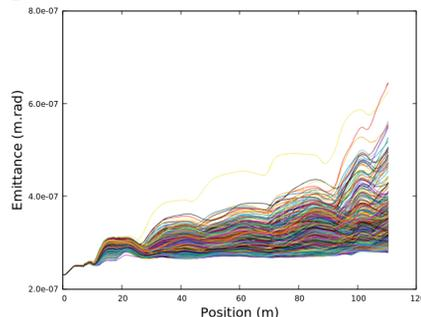
Figure 3: The Y direction emittance results in the errors and correction scheme study.
