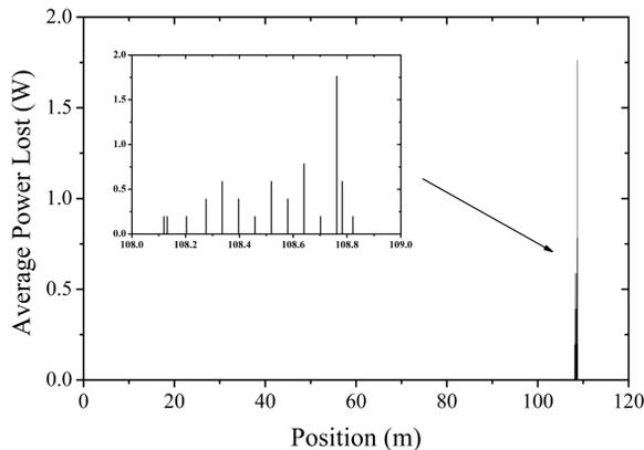
Figure 9: The average loss power along the linac and zoom in plot around the particle loss region.
