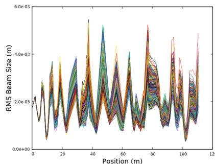
Figure 6: The Y direction rms beam size results in the errors and correction scheme study.
