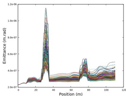
Figure 2: The X direction emittance results in the errors and correction scheme study.
