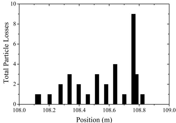
Figure 8: The total particle losses during 1000 linacs shown in different position.
