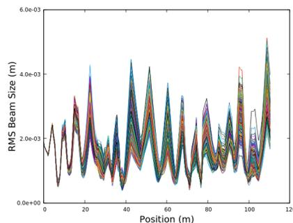
Figure 5: The X direction rms beam size results in the errors and correction scheme study.
