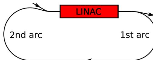
Figure 1: A layout of the double-pass proton linac [2].
