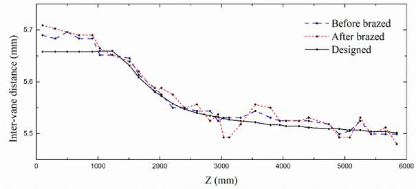
Figure 2: The designed inter-vane distances and measured inter-vane distances before and after brazing.
