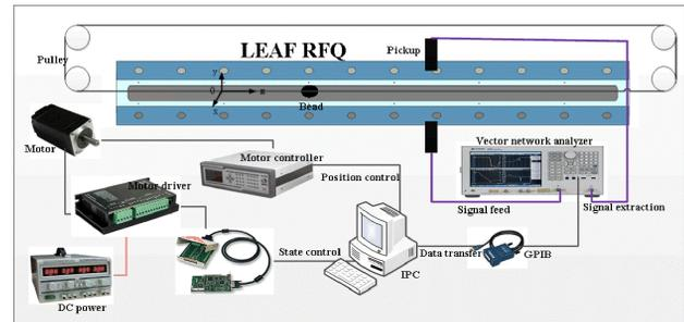
Figure 3: The sketch map of the LEAF RFQ low power test system.
