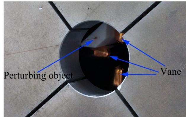
Figure 4: The teflon perturbing object used in the low power test.
