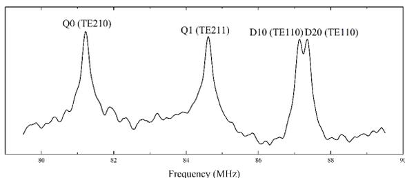
Figure 5: The measured mode spectrum in the LEAF RFQ cavity.
