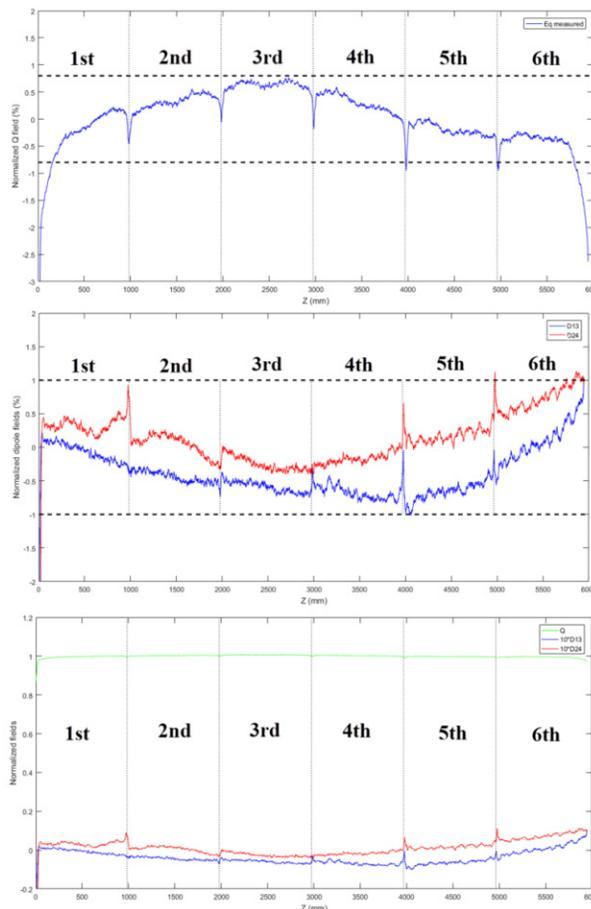
Figure 6: The longitudinal field distributions in the cavity with aluminum end-plates and copper tuners with the final depths.
