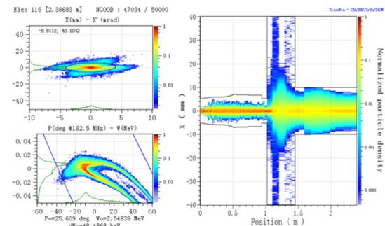
Figure 5: Particles calculation results of ADS RFQ prototype, 42.5 cm MEBT matching section together with DB-DTL prototype.
