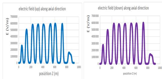
Figure 7: Electric field distribution of up/down aperture (left/right) along the cavity. With field tuning, uniform distribution is achieved.
