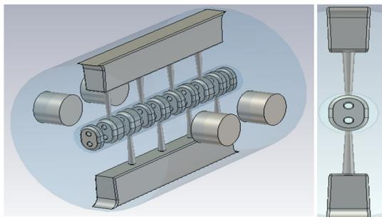
Figure 8: The structure model of IH DB-DTL, arbitrary view (left) and front view (right).
