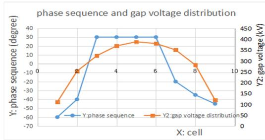
Figure 2: The phase sequence and gap voltage distribution in PIMLOC dynamics design.
