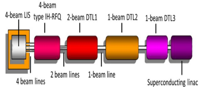
Figure 1: Simple layout of a driver system for 1 GW HIF plant. (Cited from "New development of HIF injector").
