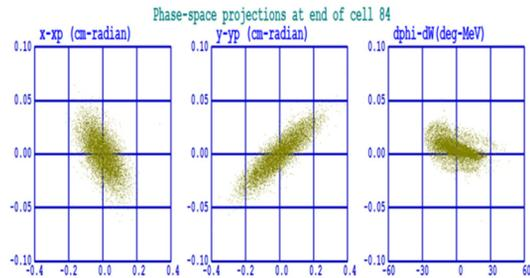
Figure 3: The emittance diagram at injection of DB-DTL.
