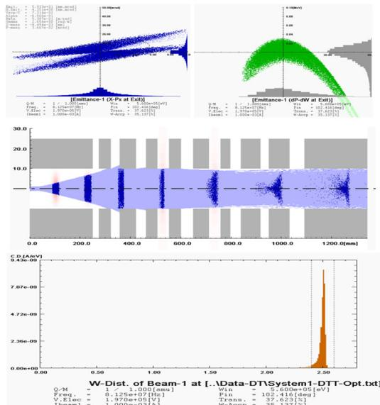
Figure 4: The emittance diagram (up: H/L) at exit of DB-DTL prototype, the beam envelop (middle), the energy spread (down) at exit of DB-DTL prototype in PiMLOC.
