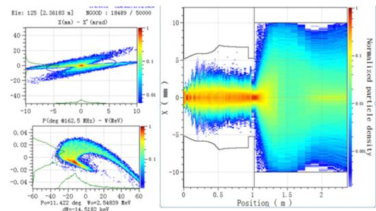
Figure 6: Particles calculation results of ADS RFQ prototype together with DB-DTL prototype.
