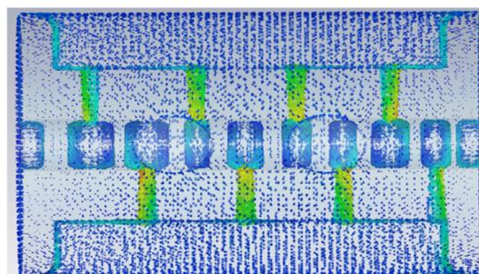
Figure 9: The surface current distribution of the cavity.
