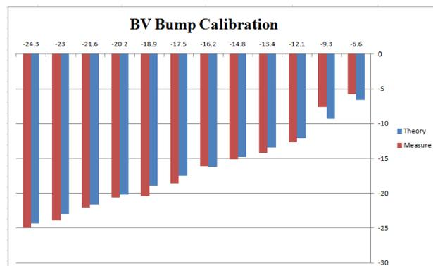
Figure 7: Comparison of the BV bump size measured in the beam commissioning and that calculated in theory.
