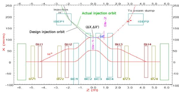
Figure 1: Layout of the CSNS injection system.
