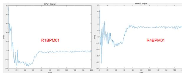
Figure 6: The turn by turn numbers measured by R1BPM01 and R4BPM01 in the experiment of BV bump calibration.
