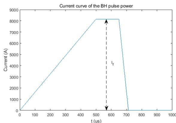
Figure 2: The current curve of the BH pulse power during the fixed injection process.
