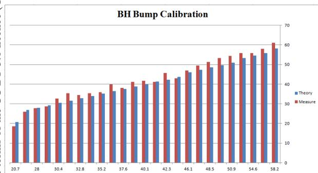
Figure 4: Comparison of the BH bump size measured in the beam commissioning and that calculated in theory.
