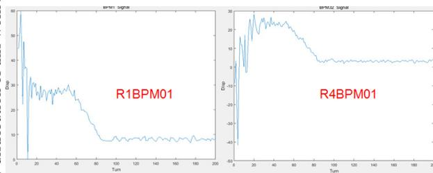
Figure 3: The turn by turn numbers measured by R1BPM01 and R4BPM01 in the experiment of BH bump calibration.
