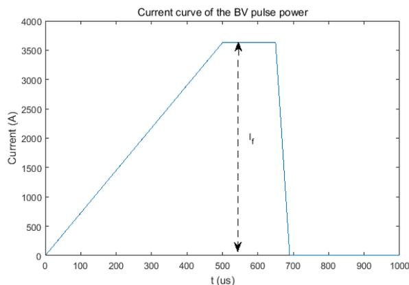
Figure 5: The current curve of the BV pulse power during the fixed injection process.
