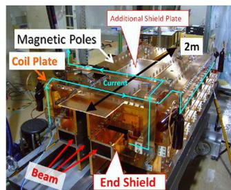
Figure 11: New low field FX septum magnet [12].
