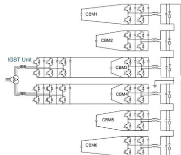
Figure 5: Circuit diagram of the dipole magnet PS.
