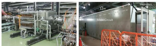
Figure 10: The injection septum magnet system developed for the high repetition rate operation: magnet in the ring (left) and power supply (right) [11].
