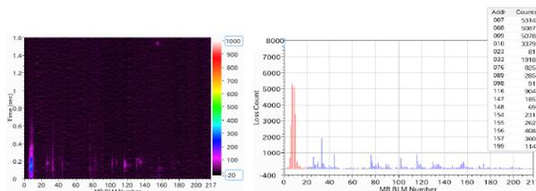
Figure 3: Distribution of beam loss monitor signal in the high power demonstration; mountain plot of one shot (left) and integrated counts (right). The sensitivity of the blue part in the right figure is eight times larger than that of the red part.
