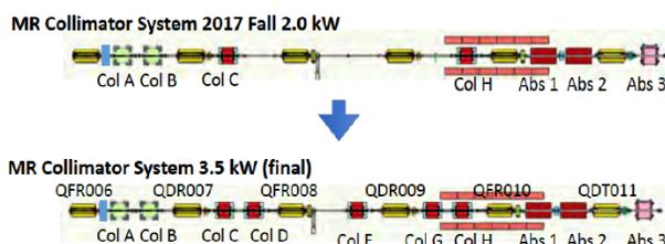
Figure 9: Configuration of the MR collimator section: present system, which has a 2.0 kW loss capacity (upper), and final system with a 3.5 kW capacity (lower).
