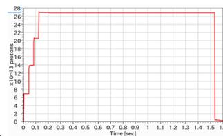
Figure 2: Circulating beam intensity in the high power demonstration.
