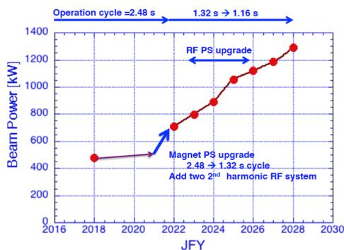
Figure 4: Power upgrade plan of the MR.
