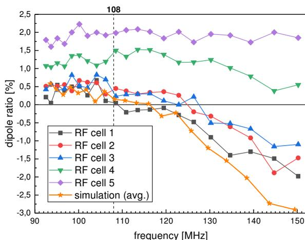
Figure 4: Measured dipole ratio in different RF cells as function of the frequency and comparison with simulation.
