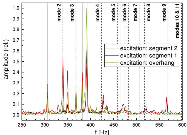
Figure 7: Measured frequency spectra of the electrode vibration amplitude for differently located excitations and comparison with simulated modes (black dashed lines) and measured resonances of the piezo mounting structure (gray lines, see Fig. 8).
