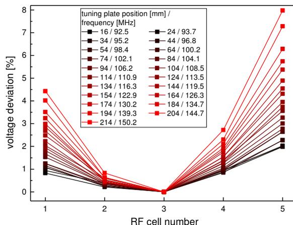
Figure 5: Measured voltage distribution along the upper electrodes (flatness) for different tuning plate positions (all at same height) / frequencies.
