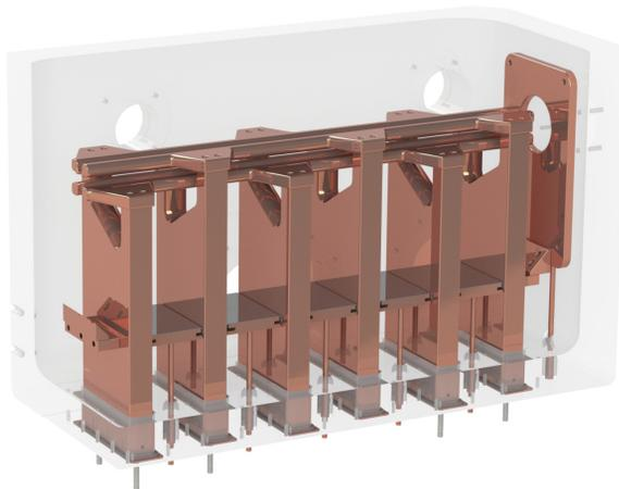
Figure 1: Rendered sectional view of the 6-stem prototype with transparent tank.
