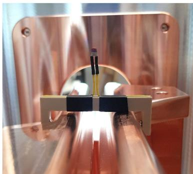
Figure 3: Perturbation capacitor (1 pF) on PEEK mounting bracket.
