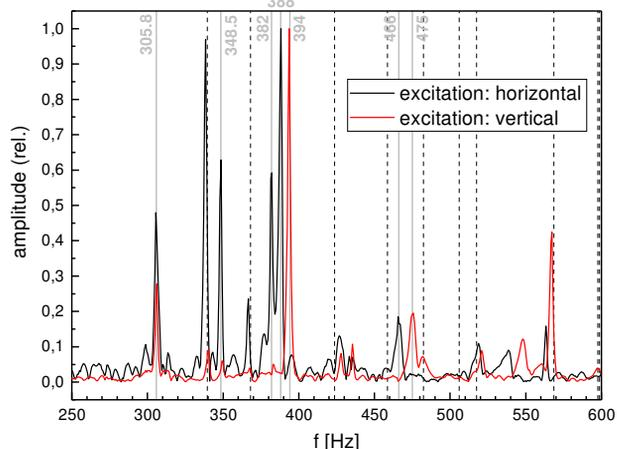
Figure 8: Measured frequency spectra for the vibration of the piezo mounting structure for horizontal and vertical excitation with the piezo pressed against the electrode.
