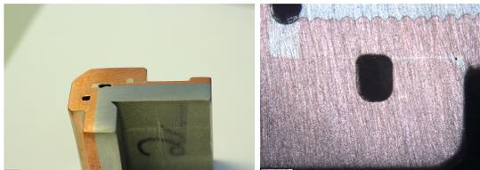
Figure 2: Close views of a cut through brazed junctions of a soldering ring, which connects the chamber's shell surface with the front surfaces.
