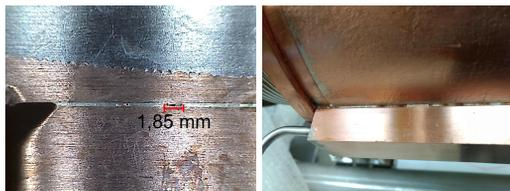
Figure 3: Close view of a cut through the junction of the cooling profile (left) and the cooling profile itself (right).
