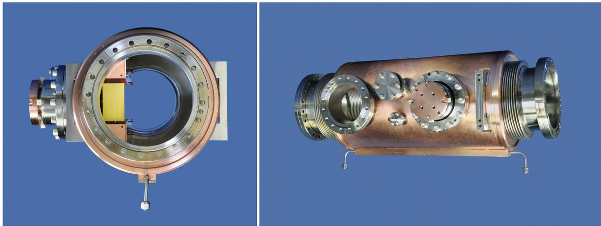
Figure 1: Photographies of the first-of-series cryocatcher. Left: Front-view, seen in beam-direction. The goldish surface catches lost beam ions. Right: Side-view, showing some features like the copper-plating of the chamber and the cooling-profile (bottom). Beam direction is from right (upstream, US) to left (downstream, DS).
