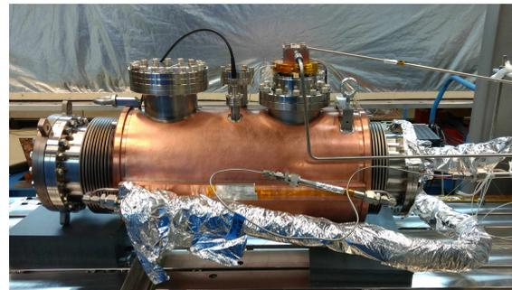
Figure 4: Cryocatcher mounted inside the universal cryostat.
