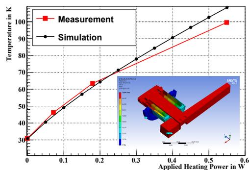
Figure 5: Temperature of the collimator block as a function of the applied additional heating power.
