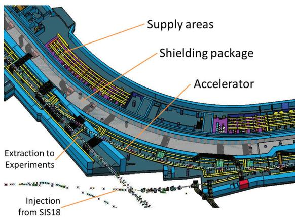
Figure 2: Detailed view of *T110* layout.
