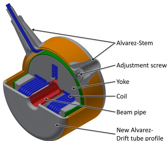
Figure 5: CAD-model of the integrated quadrupole singlet.
