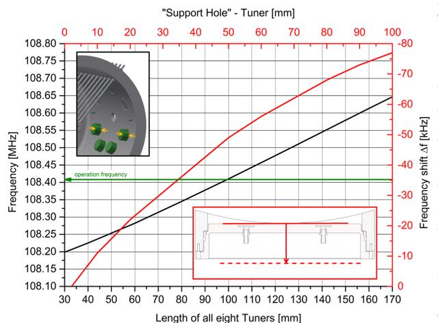
Figure 4: Simulated tuning range of the Alvarez-prototype.
