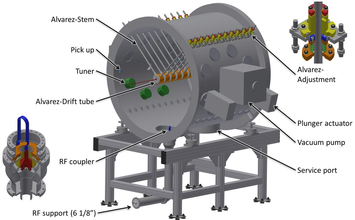
Figure 3: CAD-model of the Alvarez-FoS cavity section with a length of 1.9 m and 11 drift tubes. The drift tubes are installed at the top of the tank, but other combinations are possible. The bottom houses RF coupling, a support hole, and at the side the vacuum pumps and pickups are installed (light blue).
