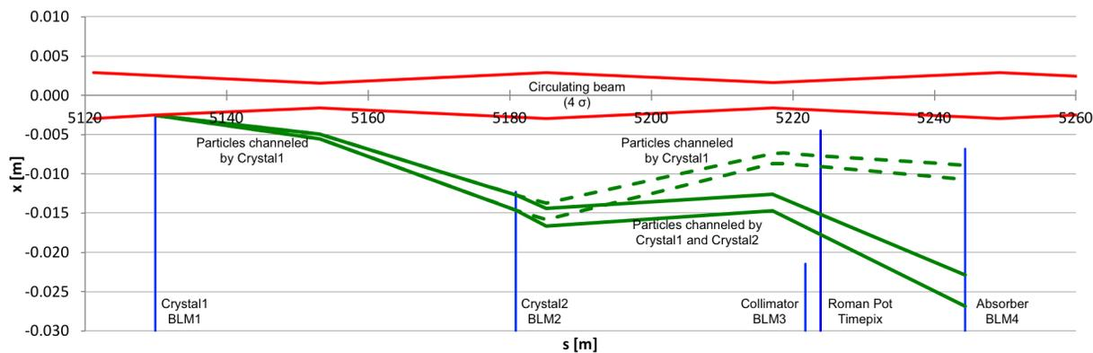
Figure 1: Horizontal beam envelope and position of the main devices in the UA9 Experiment installation.
