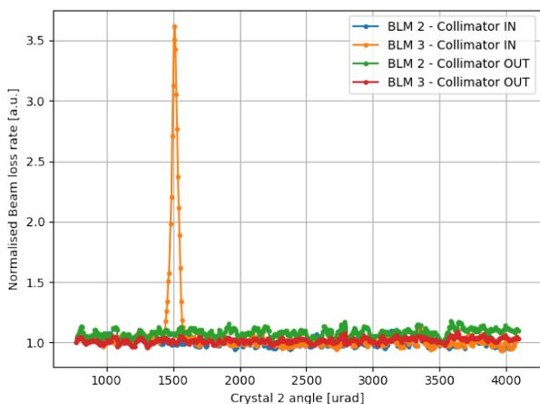
Figure 3: Beam loss rate as a function of the orientation of Crystal2 during two scans performed for its alignment.
