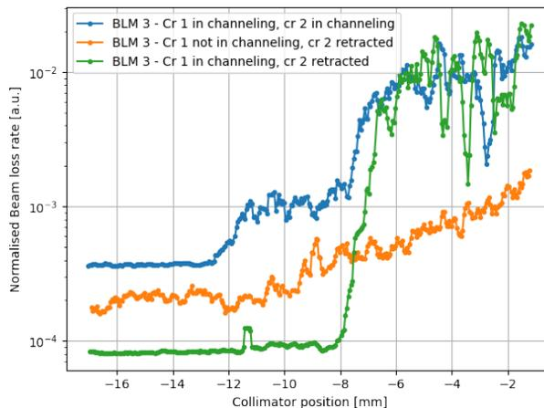
Figure 4: Beam loss rate as a function of the position of the collimator for different configurations of the crystals.
