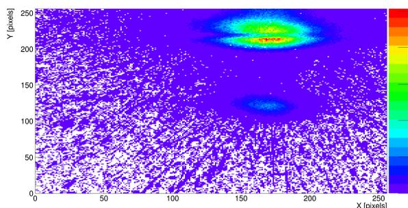
Figure 5: Image of the single-channeled (top) and double-channeled (middle) beams on the Timepix detector. The image should be rotated by  $90^\circ$  counter-clockwise in order to reproduce the real spatial position of the beams. The color scale represents the average number of counts per second per pixel.
