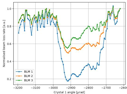
Figure 2: Beam loss rate as a function of the orientation of Crystal1 during its alignment.
