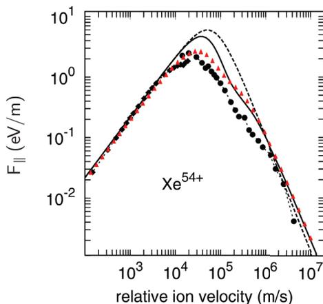
Figure 2: Longitudinal cooling force for various fully stripped  $\text{Xe}^{54+}$  ions as function of the relative ion velocity with respect to the rest frame of the electron beam. Black marks: experimental data. Solid curve: binary collision approximation. Dashed curve: empiric formula as proposed in BETACOOOL. Red triangles: simulated data with RF-Track.
