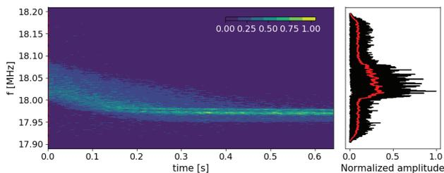
Figure 3: Schottky signal as measured at LEIR during the cooling process. The black histogram shows the power spectrum at the 50<sup>th</sup> harmonic, at 0 ms. The red curve shows a rolling average over 500 samples (<1% of the total number of samples).
