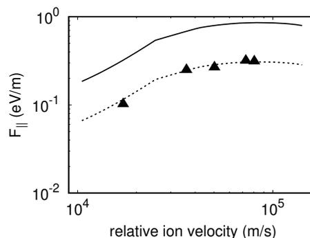
Figure 4: Longitudinal cooling force for  $\text{Xe}^{39+}$  ions at LEIR, as a function of the relative ion velocity with respect to the rest frame of the electron beam. The solid curve is the result of a simulation with nominal electron density  $n_e = 8 \cdot 10^{13} \text{ m}^{-3}$ . The dashed curve is a simulation with  $n_e = 5 \cdot 10^{11} \text{ m}^{-3}$ . The markers are the measured points.
