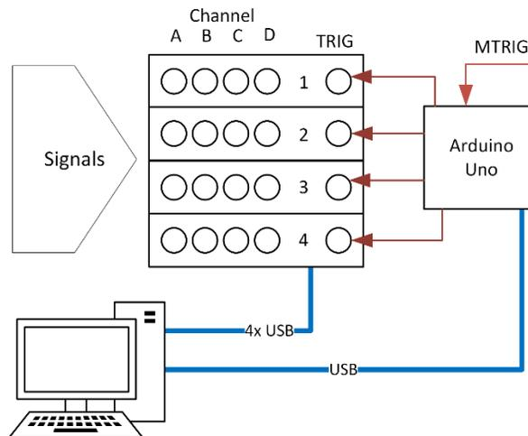
Figure 2: Pulse-by-pulse acquisition system.
