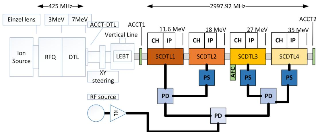
Figure 1: Actual layout of the TOP-IMPLART linac with the medium energy booster section in colors.
