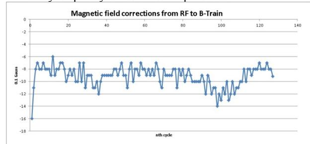
Figure 3: Corrections sent to the B-train cycle per cycle during a treatment from the minimum to the maximum carbon beam energy.
