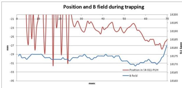
Figure 2: Position in a dispersive pick-up and magnetic field during the injection: 0 msec is when beam is injected in the ring, 20 msec is the start of the RF adiabatic voltage ramp; 60 msec is the beginning of the acceleration.
