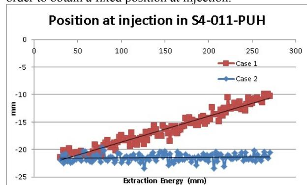
Figure 4: Comparison of the position at injection when the B field corrections are calculated by a dispersion that depends or does not depend on the extraction energy.
