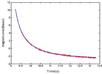
Figure 1: Trend of the magnetic field error after the dipole has reached 2990 A without B-Train feedback.
