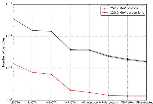
Figure 2: Intensities throughout the accelerator.
