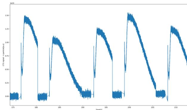
Figure 3: Main ring current transformer measurements. The effect of cycle shortening is visible on the spills where only a fraction of the intensity is required.
