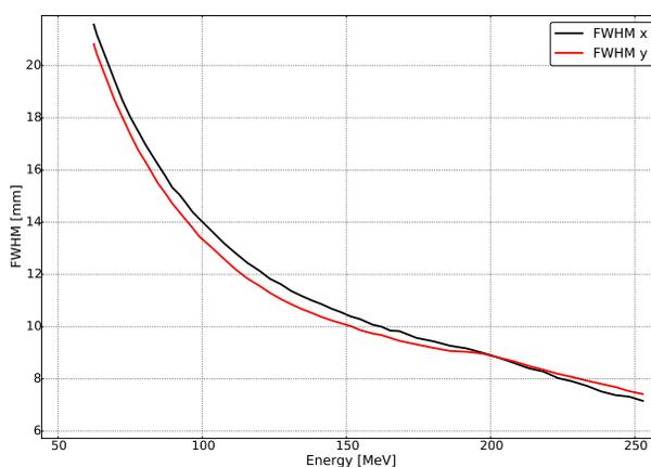
Figure 1: FWHM measured for 50 energies at the isocenter of IR2-V.
