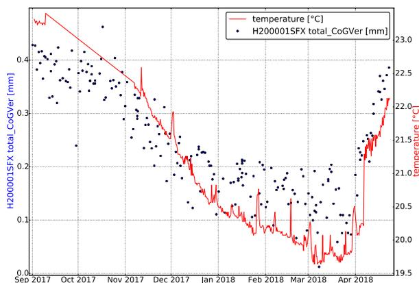
Figure 5: Position changes in the transfer line and temperature variations over several months.
