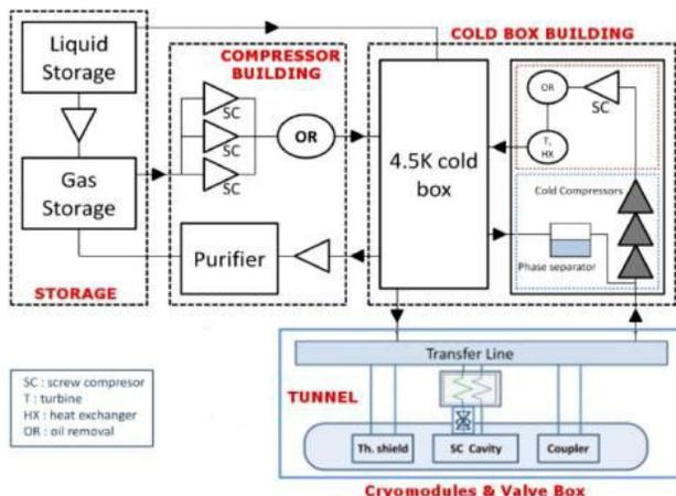
Figure 2: Cryogenic refrigerator configuration.
