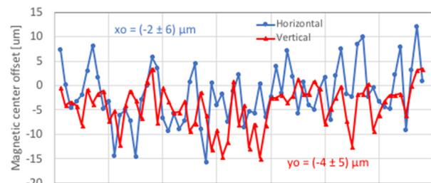
Figure 4: Magnetic centre measurements of Sirius storage ring quadrupoles Q14.
