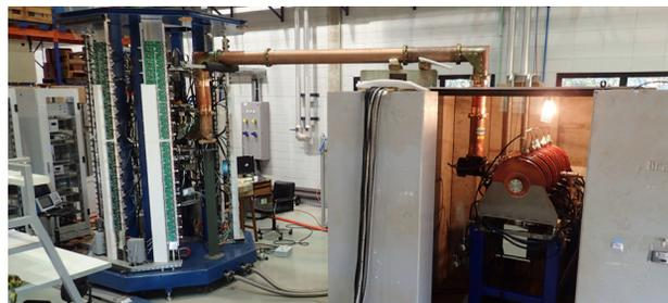
Figure 5: Setup for RF conditioning of the booster 5-cell Petra cavity with 500 MHz SS amplifiers.
