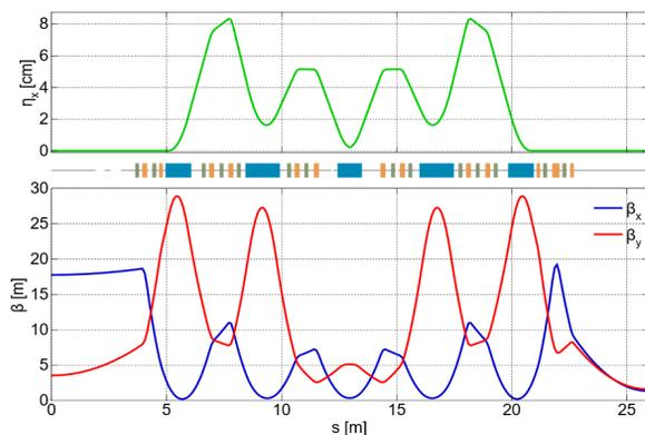
Figure 3: Optical functions for Sirius with 1/2 high beta straight to the left and 1/2 low beta straight to the right.
