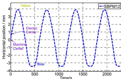
Figure 9: Beam position in SBPM12 throughout the entire time period.
