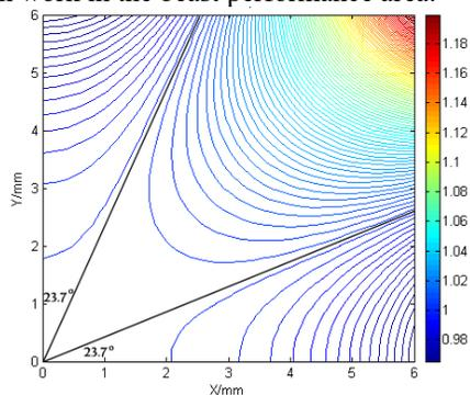
Figure 2: Simulation results of the ideal SBPM probe.
