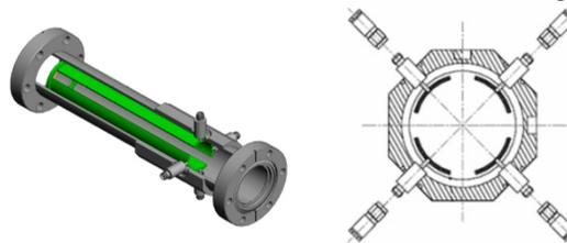
Figure 1: 3D model and section structure of SBPM.
