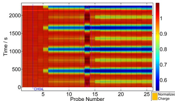
Figure 10: The normalized sum signal changes for all SBPMs collected in one hour.
