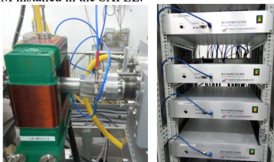
Figure 3: The installed SBPM and DBPM.
