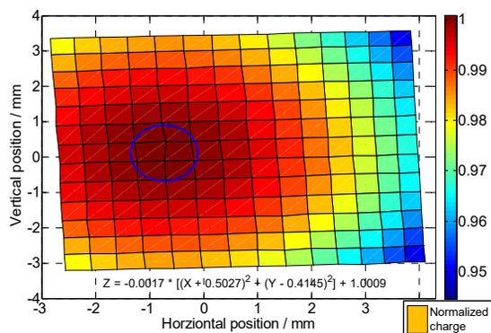
Figure 7: Results of the deviation between the electrical center and the mechanical center of SBPM11.
