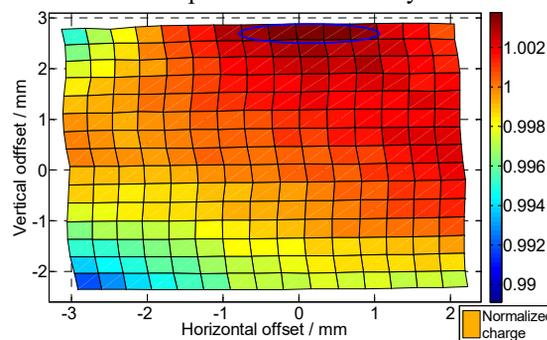
Figure 6: Results of the deviation between the electrical center and the mechanical center of SBPM7.
