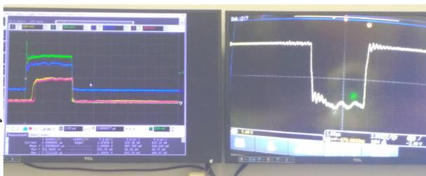
Figure 3: The electron beam current along accelerator (left photo, green line is FCT 1 pulse, blue line FCT 2, yellow is FCT 4, purple is FCT 5) and at the Faraday cup at the Neutron generating target (right photo).
