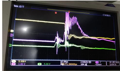
Figure 6: Thyatron circuit RF ringing. Purple and green lines are thyatron grid ringings. Yellow line is thyatron anode voltage ringing.
