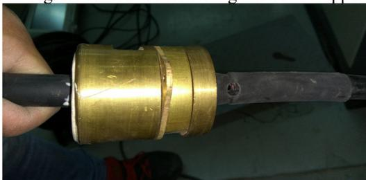
Figure 5: The example of the HV voltage cable breakdowns.
