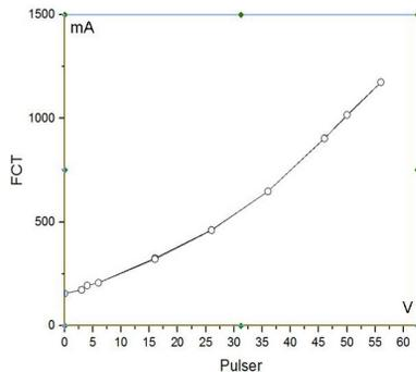
Figure 4: Triode electron gun current vs grid pulser voltage. Bias voltage is 50 V.
