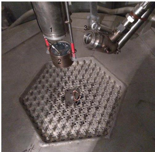
Figure 2: Testing beam instrumentation equipment at the end of the NSC KIPT SCA Neutron Source: 1 is stainless steel pipe with alumina window, 2 is lead Faraday cup, 3 is CCD camera.
