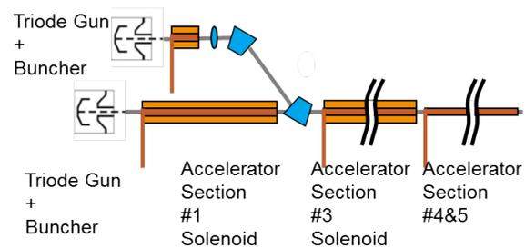
Figure 7: Overview of the replacement of the bombarder gun with the triode gun.
