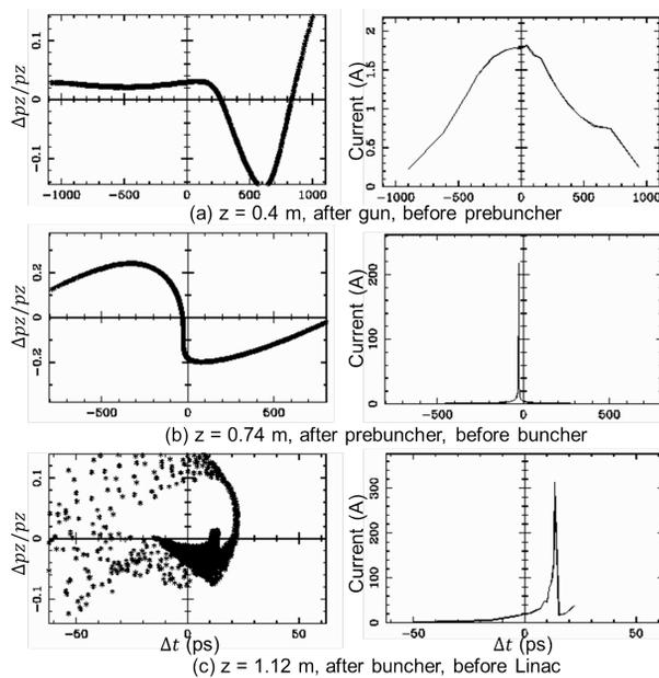
Figure 4: Longitudinal distribution of the electrons in different  $z$  position.
