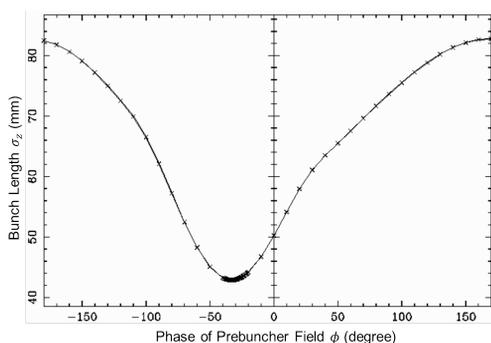
Figure 3: The electron bunch length after prebuncher versus the phase of the prebuncher electric field, calculated in ASTRA.
