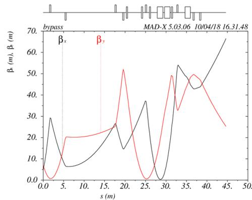
Figure 6: The twiss parameters along the PIA bypass calculated in MADx.
