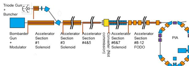
Figure 1: Overview of the current injection system of the Linac II and PIA.
