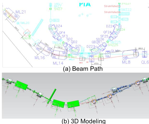
Figure 5: The drawing of the PIA bypass:(a) AutoCAD designed beam path, the bypass is shown in red, and (b) the NX 3D modeling of the bypass optics.
