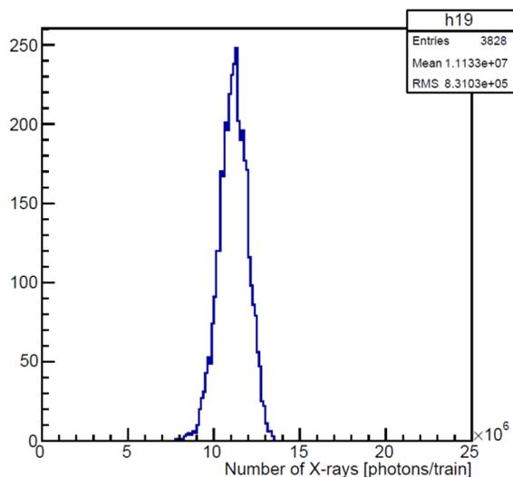
Figure 2: Histogram of LCS X-ray flux measurement. Flux are measured by each macro pulses.
