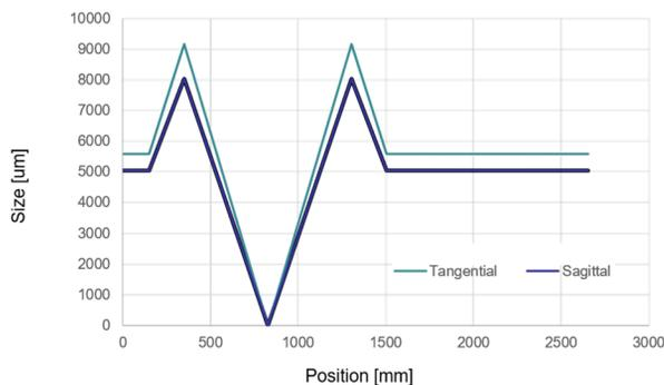
Figure 6: Calculated cavity mode profile in the 6 mirrors optical cavity using 2 plane mirrors, 2 convex mirrors and 2 concave mirrors.
