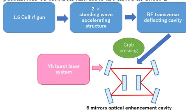
Figure 4: Schematic illustration of the upgraded LUCX facility.
