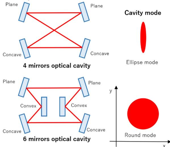
Figure 5: Comparison of 4 mirrors optical cavity and 6 mirrors optical cavity. The cavity forms are on the left and its cavity modes are on the right.
