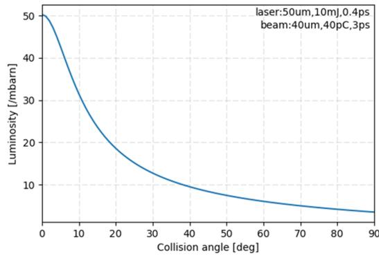
Figure 3: Luminosity as a function of collision angle.
