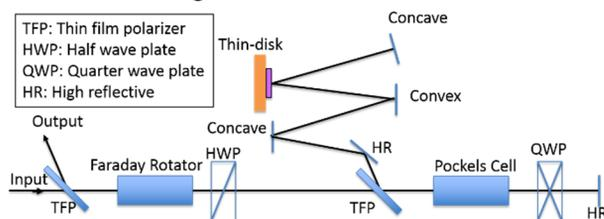
Figure 9: Schematic of thin-disk regenerative amplifier.
