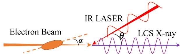
Figure 5: Schematic of crab crossing LCS.
