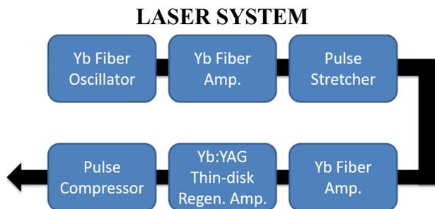
Figure 8: Schematic of laser system.
