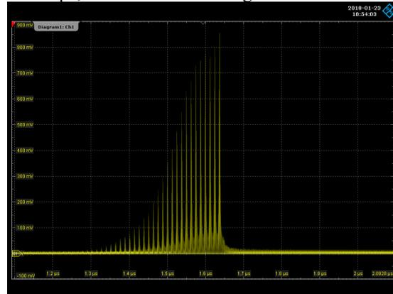
Figure 10: Pulse build-up in regen amplifier.
