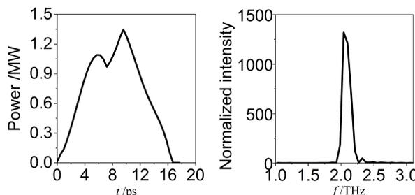
Figure 6: Time structure (left) and the output FEL pulse (right) for 2.0 THz.
