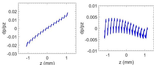
Figure 4: Energy spread at gun exit (left) and at undulator entrance (right).
