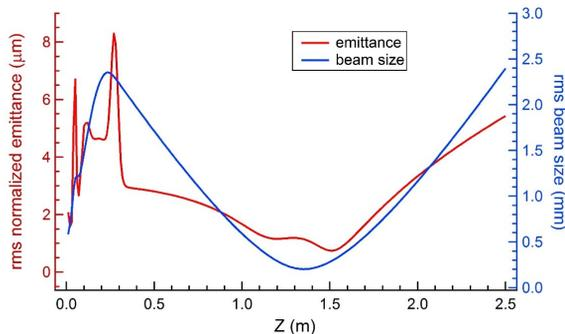
Figure 3: Evolution of transverse emittance and beam size of HALS beam
