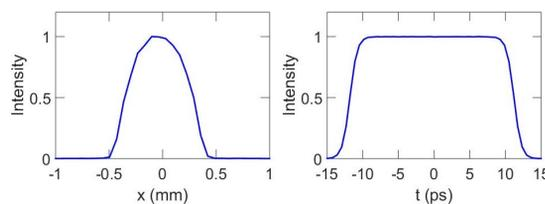
Figure 4: transverse (left) and longitudinal (right) beam profile of the electron source
