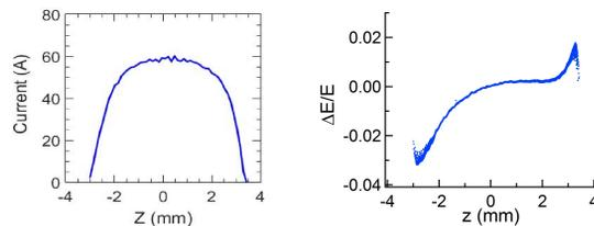
Figure 6: Beam current profile (left) and energy spread profile (right)
