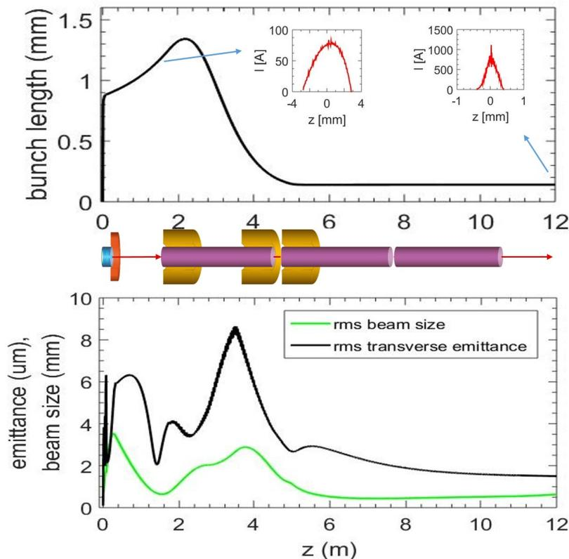
Figure 7: Simulation results of BAVB scheme. The top plot shows the rms bunch length evolution with current profiles before and after compression posted. The bottom plots are the transverse emittance and rms beam size.
