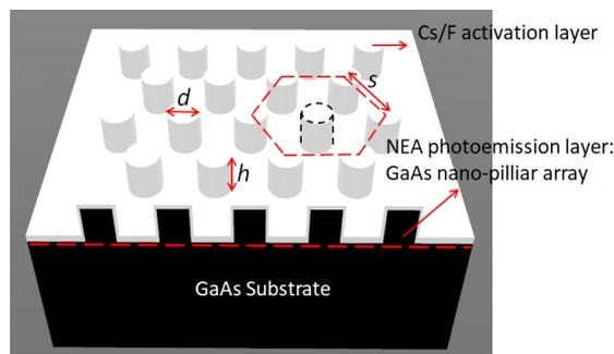
Figure 1: Illustration of structure of a NEA GaAs photocathode device.
