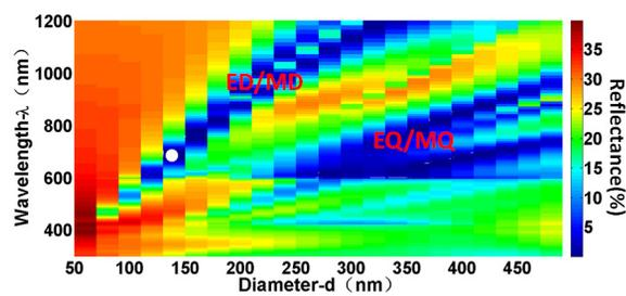
Figure 3: Predicted surface reflectance spectra for GaAs NWA structures as a function of nanowire diameter ( $d$ ), where height ( $h$ ) and spacing ( $s$ ) were set to 500nm and 600nm, respectively.
