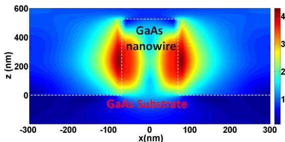
Figure 4: A plot of the electric field intensity ( $|E|^2$ , colour scale) as a function of position along the photocathode surface, showing the simulated dipole resonance mode profile within a vertical cross section of the GaAs nanowire resonator on the GaAs substrate ( $d = 140$  nm and  $\lambda = 727$  nm) in the plane parallel to the E-field of the linearly polarized incident light.
