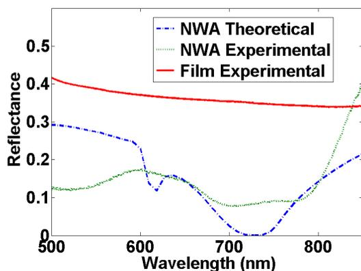
Figure 5: Measured and predicted surface reflectance spectra for GaAs photocathode with and without the NWA resonator (the dimensional parameters:  $d = 140$  nm,  $h=525$ nm and  $s=600$ nm).
