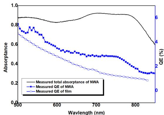
Figure 6: Measured light absorption together with QE for GaAs photocathodes with and without the NWA resonator structure.
