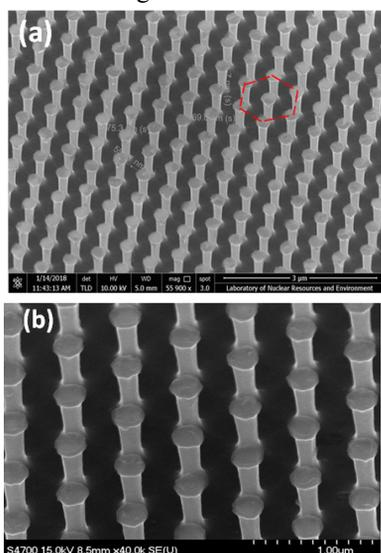
Figure 2: SEM images of the regular hexagonal GaAs NWA fabricated by SCIL: (a) Before heat clean or activation; (b) After heat clean or activation.
