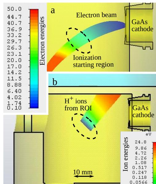
Figure 2: The region within the electrode chamber where the electron beam reaches sufficient energies to ionize molecular hydrogen (a). Ions originating from this ROI travel back a different path than the electrons and miss the GaAs cathode (b), presuming they have no initial kinetic energy.
