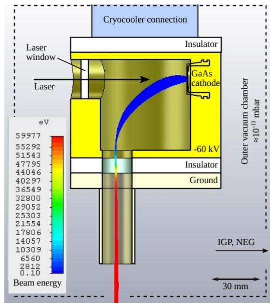
Figure 1: Simulation of the electron beam with a first layout of the cryogenic source (CST studio suite®).
